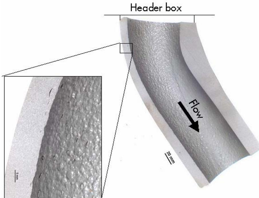
**Figure 6.** Cross-section of a bend of air cooler outlet pipe, showing the position of maximum wall loss and the presence of blisters in the pipe wall.
