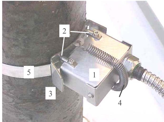
**Figure 2.** Picture of a PEC sensor (1) that is attached with a spring (4) to a frame (3). The sensor has three sharp pins (2) that fit holes in the frame.
