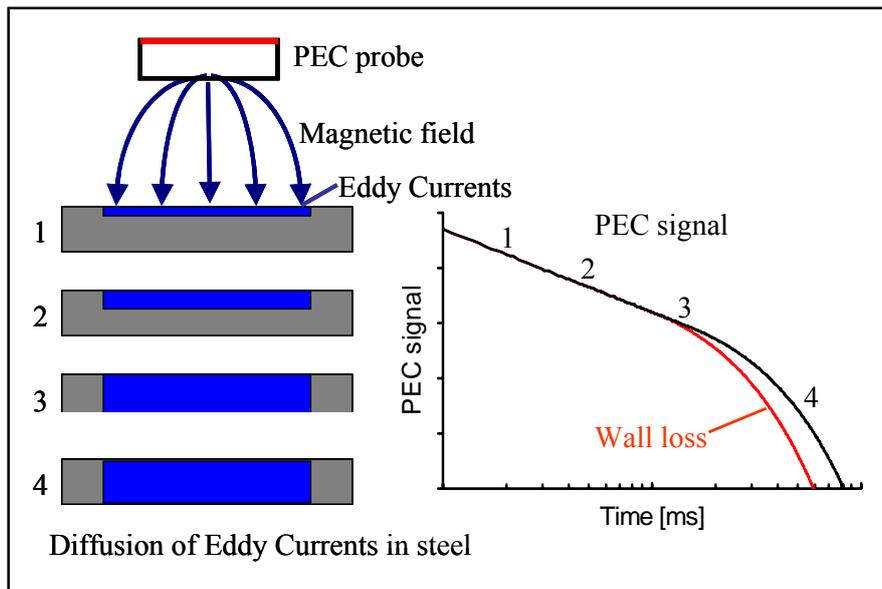
**Figure 1.** Schematic representation of diffusion of eddy currents in the steel
