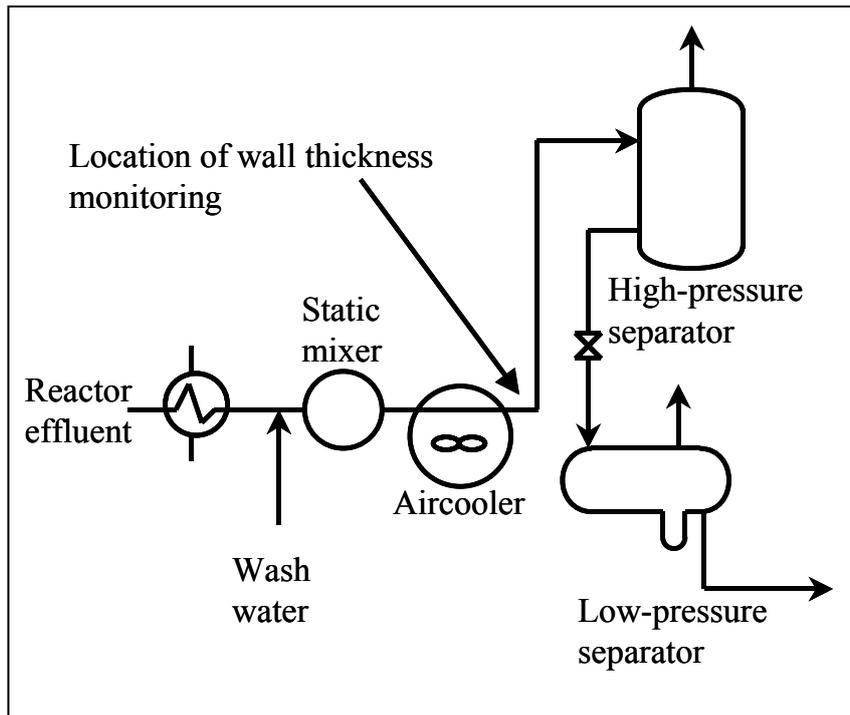
**Figure 3.** Simplified process flow diagram of the reactor effluent portion of a hydrocracker unit at a refinery
