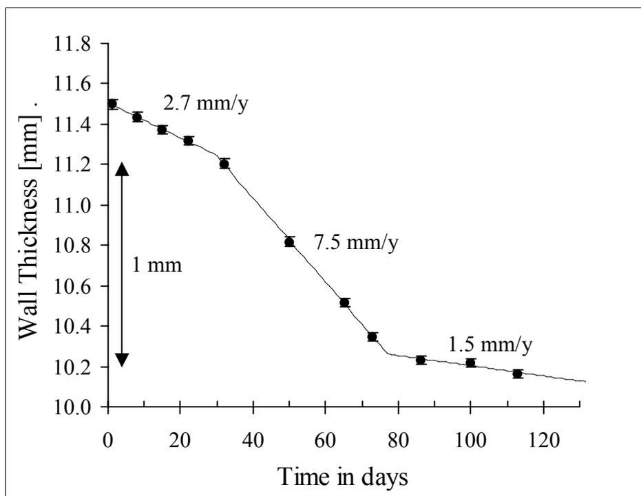
**Figure 4.** Example of a PEC result recorded on one of the outlet pipes. Note the expanded scale on y-axis.  $2\sigma$  measurement error bars are indicated.
