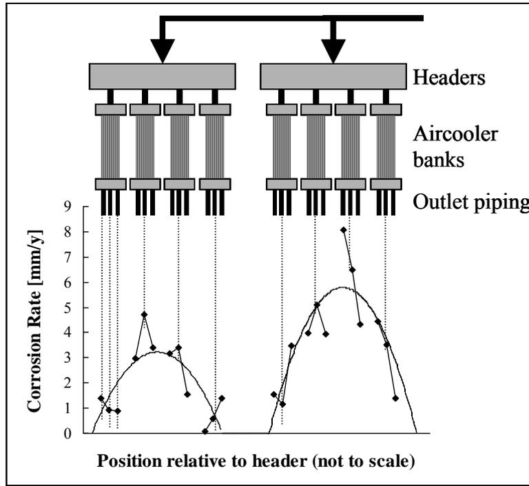
**Figure 5.** Corrosion rates measured by PEC at the 24 outlet pipes over the first 8 air cooler banks. The dashed lines indicate which pipe corresponds to which data point. The full curves serve to guide the eye to the average rate in each air cooler.
