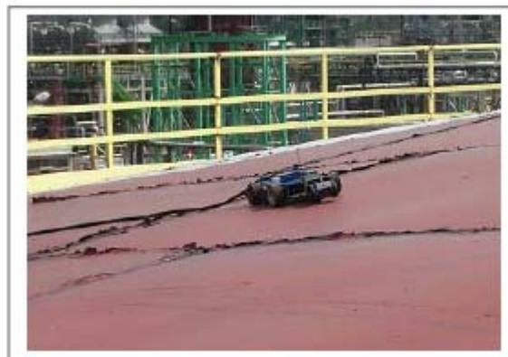
Figure 7: UT remote inspection of a tank roof (Scorpion system)
