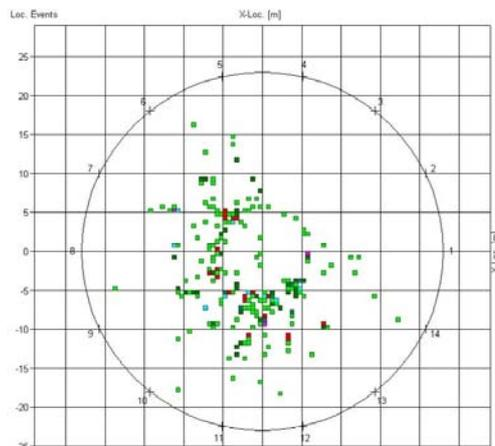
Figure 5 : results obtained by AE on a tank bottom exhibiting minor damages
