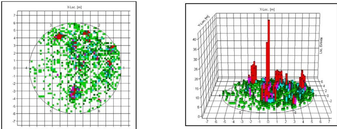
Figure 4 : results obtained by AE on a tank bottom exhibiting major damages
