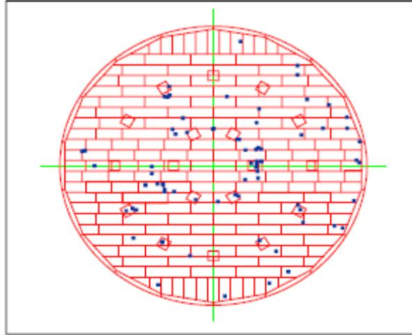
**Figure 6:** results obtained by MFL on the same tank (see figure 5)
