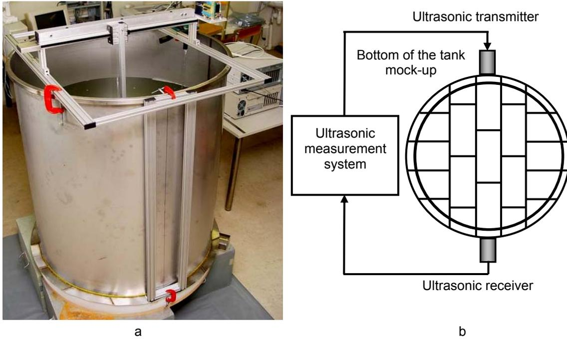
**Fig. 3.** Photo of the 1:8 scaled down size tank mock-up (a) and the measurement set-up (b) used for investigation
