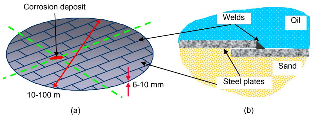
**Fig. 1.** The typical geometry of a tank floor (a) and the model of a lap joint weld (b)
