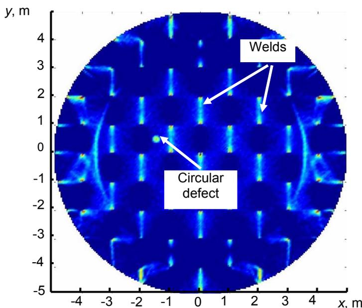
**Fig. 2.** Reconstructed ultrasonic image of the petroleum tank floor with a circular defect (from simulated data) using the through transmission tomography technique
