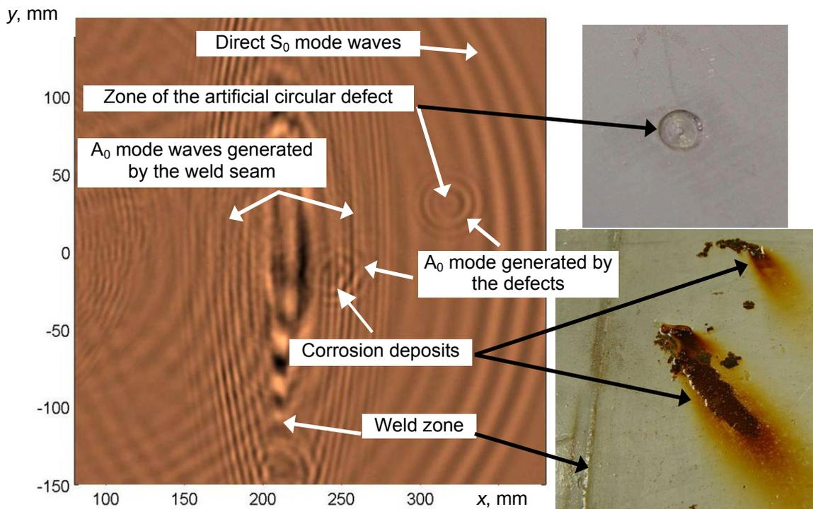
**Fig. 5.** The horizontal cross-section (at time instance  $t = 85 \mu\text{s}$ ) of the measured leaky ultrasonic field over the weld and the defects at the segment of the tank bottom plate, one of them was artificially drilled (diameter 5mm, depth 0.5 wall thickness) and another was caused by natural corrosion. The receiving transducer was placed at the distance over the plate  $z = 15 \text{ mm}$  and oriented at the  $90^\circ$  angle with respect to the horizontal plane.
