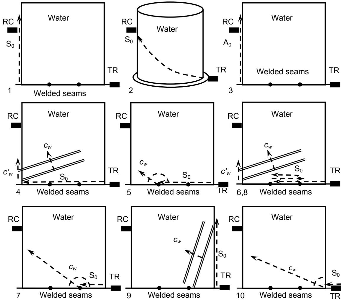
**Fig 6.** The explanation of different acoustic paths of the Lamb waves radiated into the liquid and picked-up on the vertical wall of the tank, TR denotes the transmitter and RC denotes the receiver, which was scanned vertically on the tank wall
