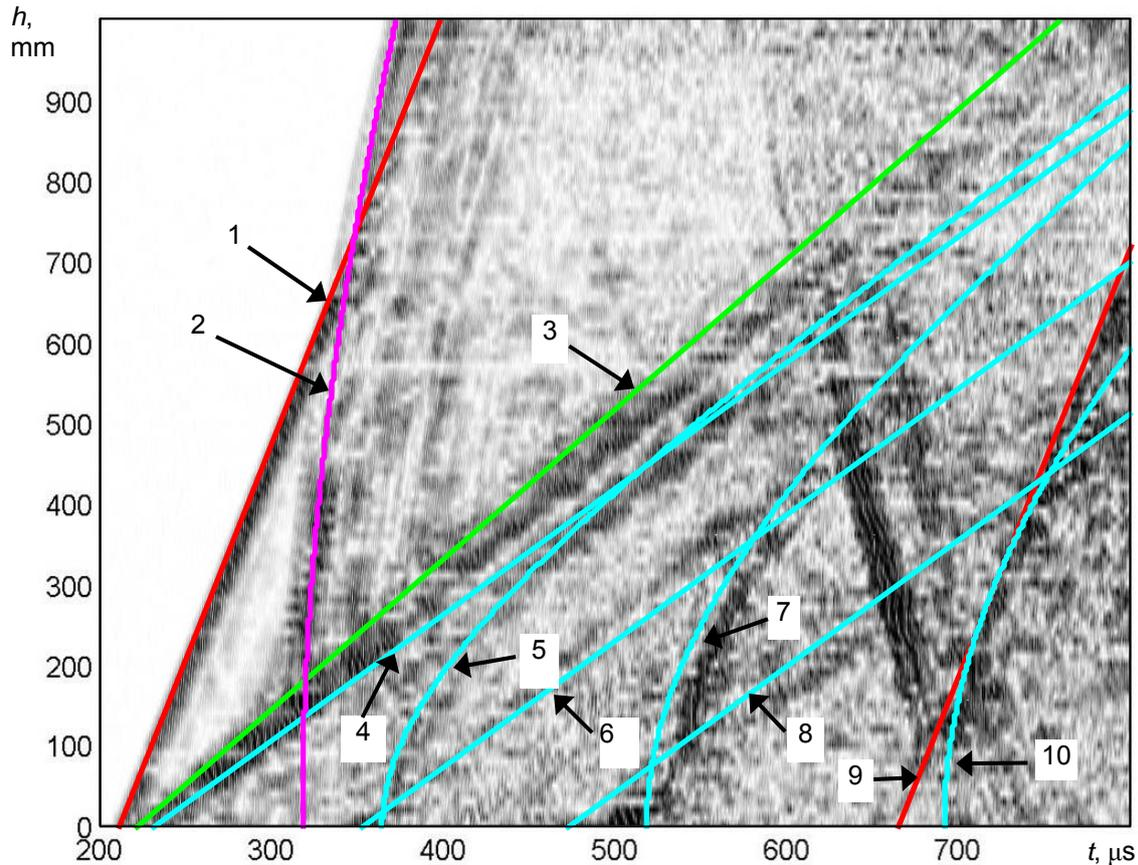
**Fig 7.** Identification of the experimentally measured waves, which were picked-up on the vertical wall of the tank. The numbers 1 - 10 correspond to the numbers in Fig.7.
