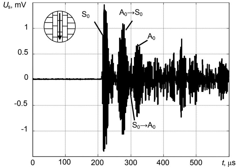
**Fig. 4.** Signal transmitted through the loaded floor of the tank mock-up, when transmitting and receiving transducers were mounted on the edges of the tank floor (flanges)
