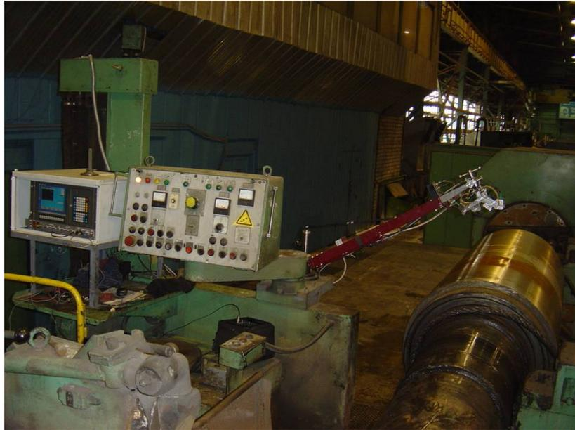
**Figure 2.** Demas Ltd. (Russian Federation) automatic ultrasonic roll-scanning system.
