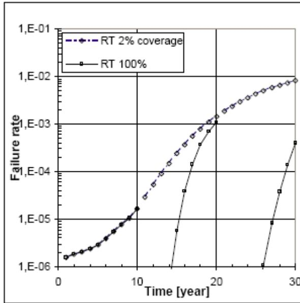
Figure 15: Effect of coverage on the failure rate
