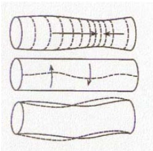
Figure 4: Wave modes in pipe
