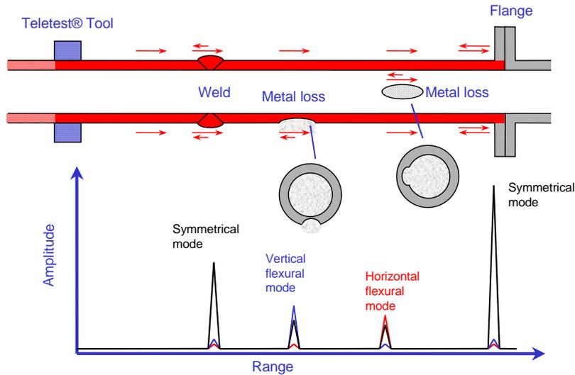
Figure 6: Types of reflected signals
