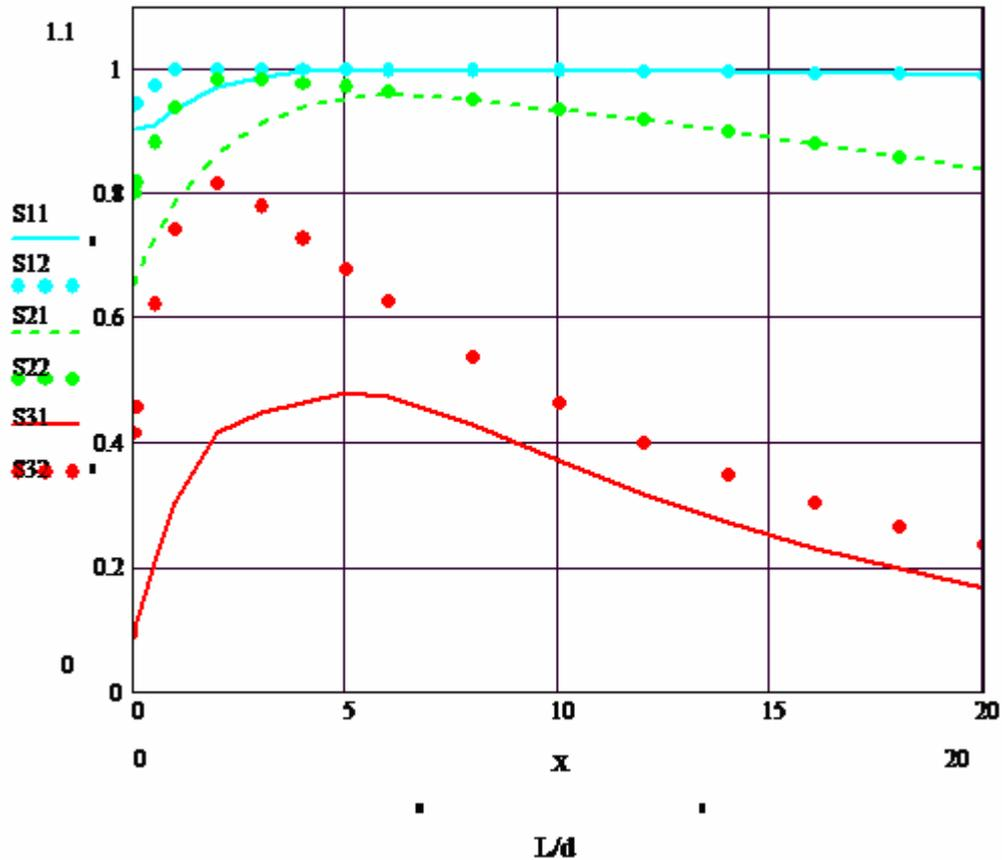
Fig. 1. Influence  $\lambda = L/d$  for cylinders made of “soft” (S11, S12), “medium” (S21, S22) and “stiff” (S31, S32) materials according to the Table 1 on the sensibility  $S_{H_{cs}}^{M_d}$  of the informative control parameter  $M_d$  to  $H_c$  of the materials at magnetizing of cylinders in an open magnetic circuit in an external field  $H_e = 60$  kA/m (S11, S21, S31) and 200 kA/m (S12, S22, S32).
