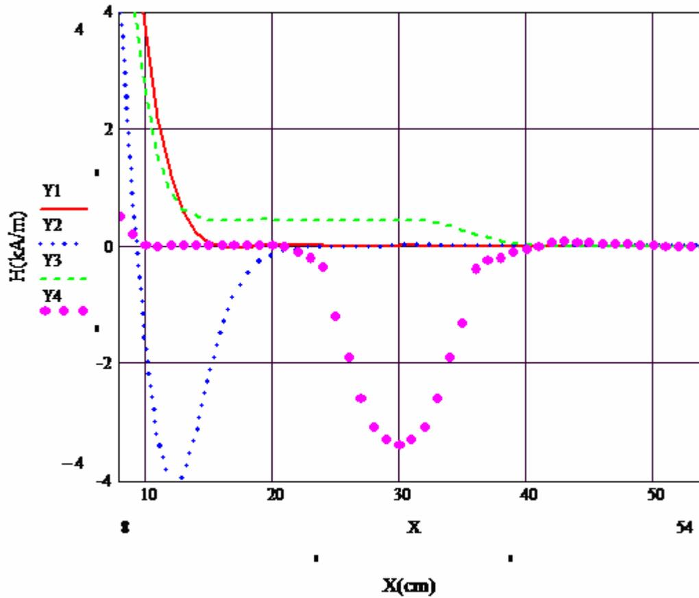
Fig. 4. Possible distributions of the magnetic field along the axis of the products motion in the control region.
