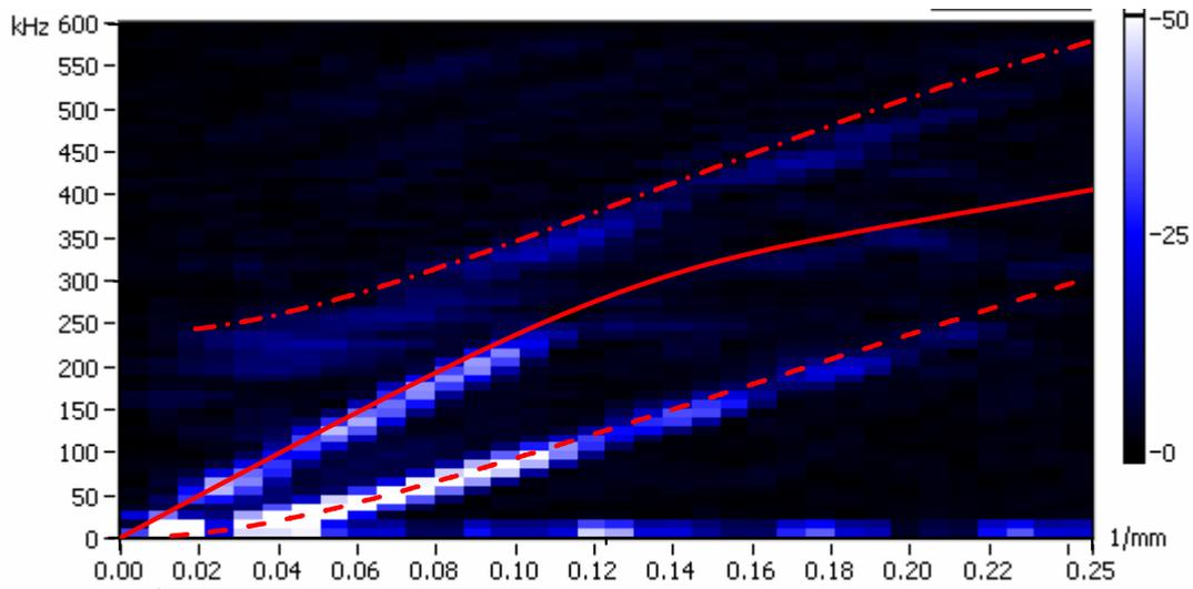
**Figure 10.** Dispersion map with the calculated dispersion curve swapped; solid line S0, dashed line A0, dashed-dotted line A1; the parameters for the calculation were:  $c_l = 2.73 \text{ mm}/\mu\text{s}$ ,  $c_t = 1.43 \text{ mm}/\mu\text{s}$ ,  $d = 3 \text{ mm}$ .
