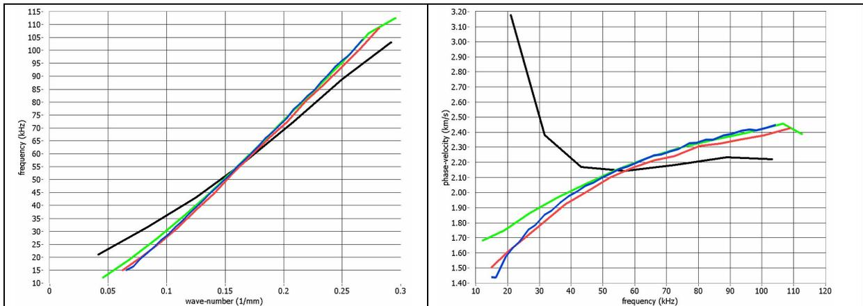
**Figure 15.** Dispersion diagram of the phase velocity calculated out of the dispersion maps generated with different line length. Left: Frequency versus wave number. Right: Phase velocity versus frequency. The length of the evaluation line amounts for the blue, red, green and black line 85, 65, 45, and 25 mm, respectively.
