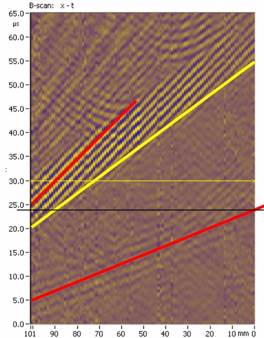
**Figure 3.** B-scan along the horizontal (green) line of Figure 2 ( $y = 30 \text{ mm}$ ).
