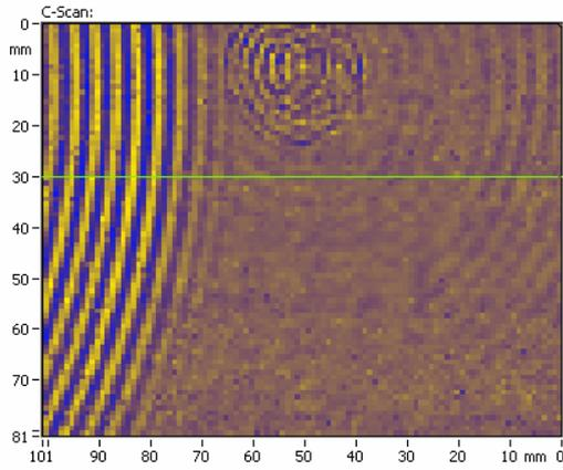
**Figure 2.** C-scan (snapshot of the wave field) at  $t = 30 \mu\text{s}$ , the horizontal and the vertical axis are given in mm.
