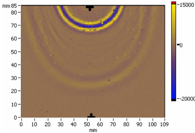
**Figure 13.** Snapshot of the wave field on a triax GFRP plate.  $t = 50 \mu\text{s}$
