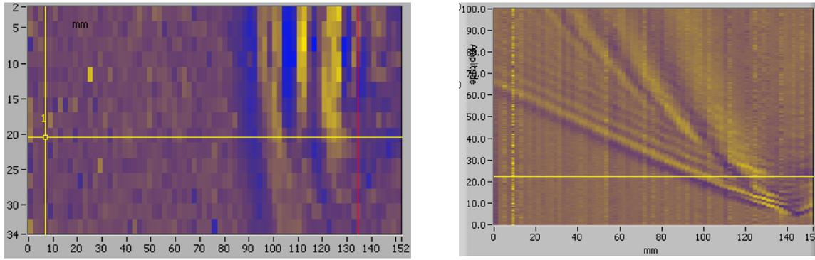
**Figure 8.** Snapshot (left) and B-scan (right) of the wave field generated by a piezoelectric fiber patch into a Perspex plate of 3 mm thickness.
