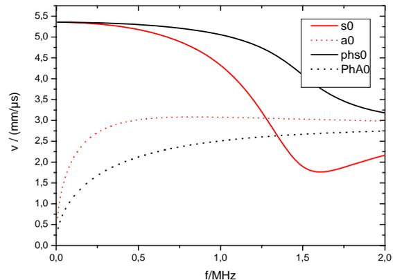
**Figure 5.** Group velocity (red) and phase velocity (black) for the two lowest modes of the dispersion diagram (see [11]).
