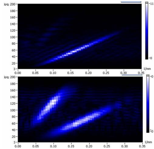
**Figure 14.** Dispersion map for the vertical line in Figure 13 connecting the two cursor positions. The signals were truncated ( $\cos^2$  filter) at  $t = 400 \mu\text{s}$  (top) and  $t = 100 \mu\text{s}$  (bottom)
