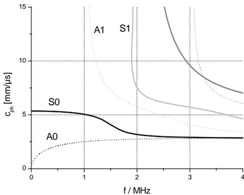
**Figure 4.** Phase velocity dispersion diagram for an aluminum plate of thickness  $d = 1.5 \text{ mm}$  (see [11]).
