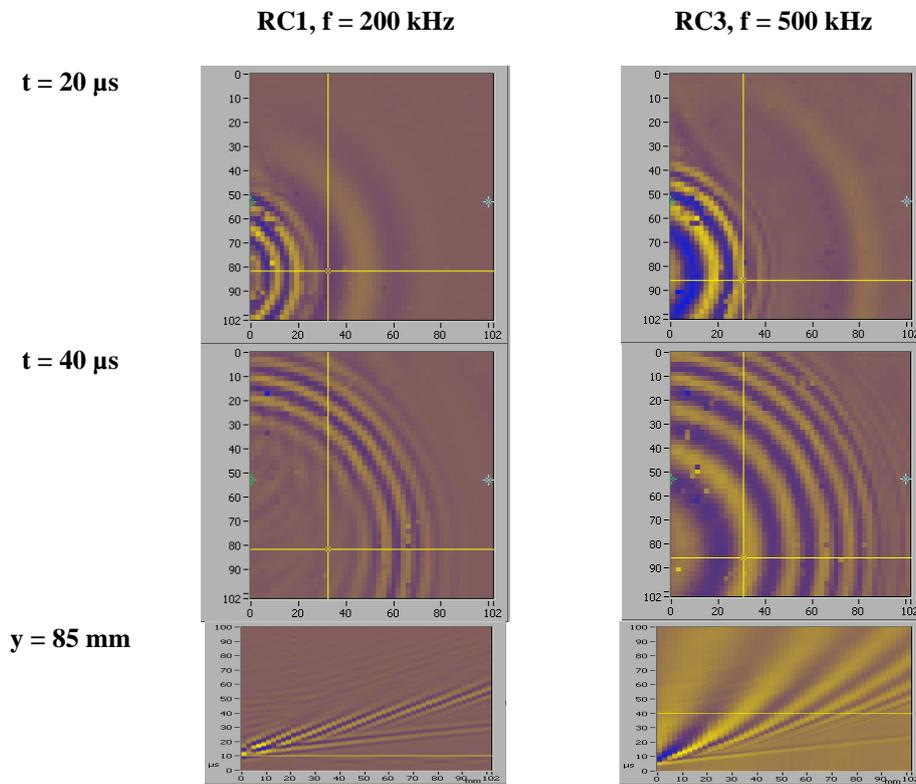
**Figure 6.** Snapshots and B-scans for different excitation conditions. Left: RC3 with  $f = 200$  kHz, right: RC 1 with  $f = 500$  kHz; upper line: snapshot at  $t = 20$   $\mu$ s, middle line: snapshot at  $t = 40$   $\mu$ s, bottom line: B-scan for a horizontal line through the excitation point (see horizontal line in the snapshots).
