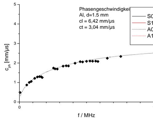
**Figure 12.** Extracted phase velocity data (points) compared with the numerical results of A0 mode (dashed curve).
