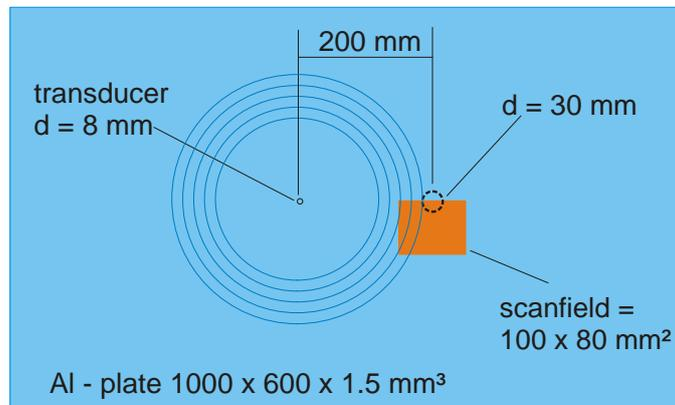
**Figure 1.** Experimental arrangement for generation and laser detection of Lamb waves in an aluminum plate.
