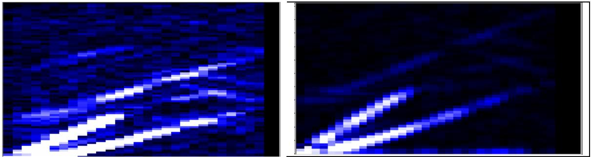
**Figure 9.** Dispersion maps of the data of Figure 8; left: from row data; right: after  $\cos^2$  filtering and averaging the measured data over 7 adjacent lines.
