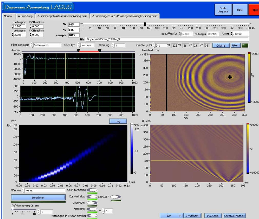
**Figure 7.** Software surface of the evaluation program. The windows contain: a snapshot of the wave motion (upper right), two time signals at cursor position selected in the snapshots (upper left), a B-scan over the line between the selected cursor positions (lower right) and the dispersion curve (lower left).
