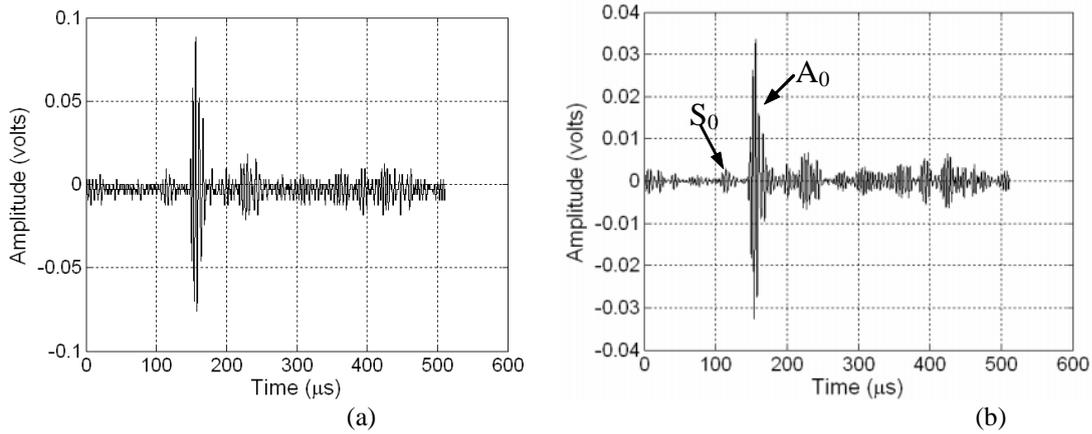
Figure 2. AE signal recorded from channel 1 (a) waveform showing distinct  $S_0$  and  $A_0$  (b) filtered signal.
