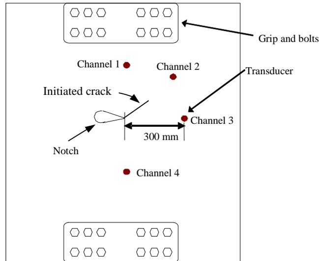
Figure 1. Fatigue test setup indicating location of sensors.
