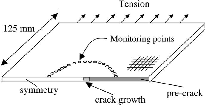
Figure 8. 3D plate model used to simulate acoustic wave from crack length growth with pre-crack.
