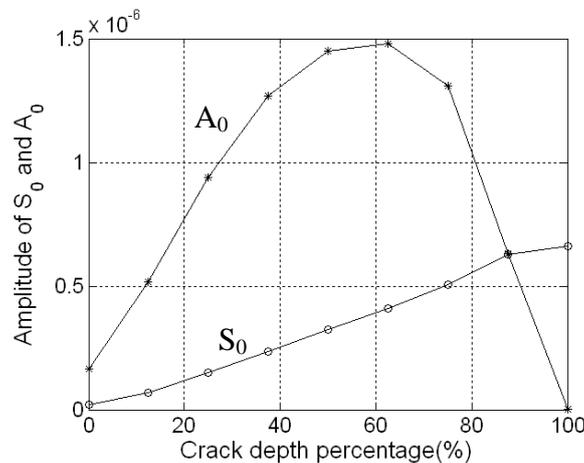
Figure 7. Collection of the amplitude of the  $S_0$  and  $A_0$  modes from different fatigue crack depths.
