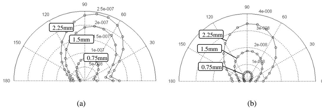
Figure 10. A polar plot showing the radiated angular mode is skewed toward the pre-crack edge: (a)  $A_0$  mode and (b)  $S_0$  mode
