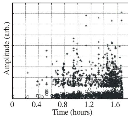
Figure 3. Amplitude of the  $S_0$  (open circles) and  $A_0$  (asterisks) modes over the duration of the fatigue test.
