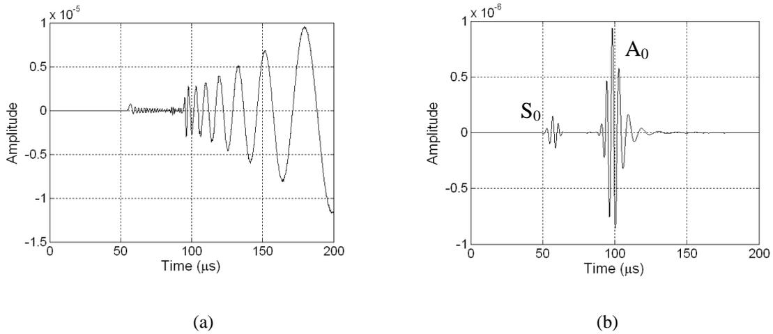
Figure 6. Typical results from FE model: (a) recorded signal from output node and (b) the signal after filtering its frequency spectrum showing separation of the  $S_0$  and  $A_0$  modes.
