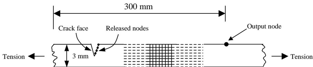
Figure 5. Cracking through the thickness of the plate.
