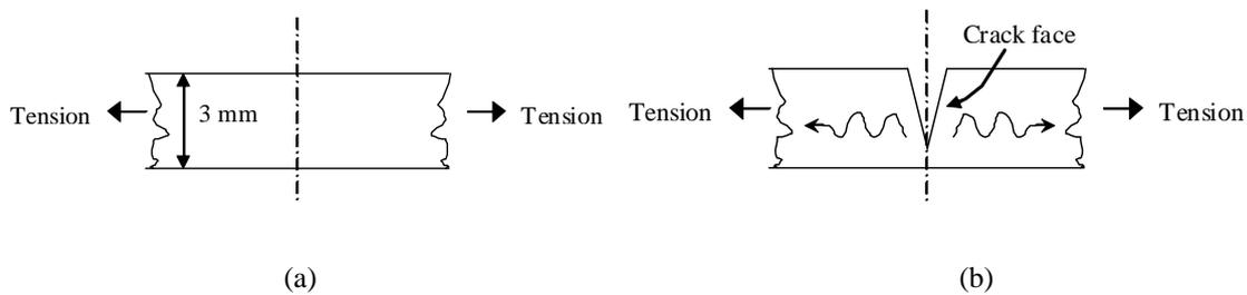
Figure 4. Crack through the thickness of the plate (a) before and (b) after crack growth.
