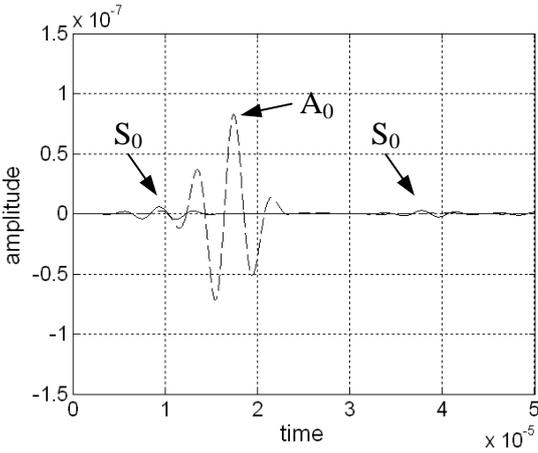
Figure 9. Added and subtracted signal showing the separated  $S_0$  and  $A_0$  modes
