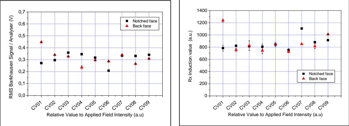
**Figure 4.** Barkhausen signal and RXI relative to induction value versus applied excitation intensity of irradiated specimens measured on two faces (100 Hz)
