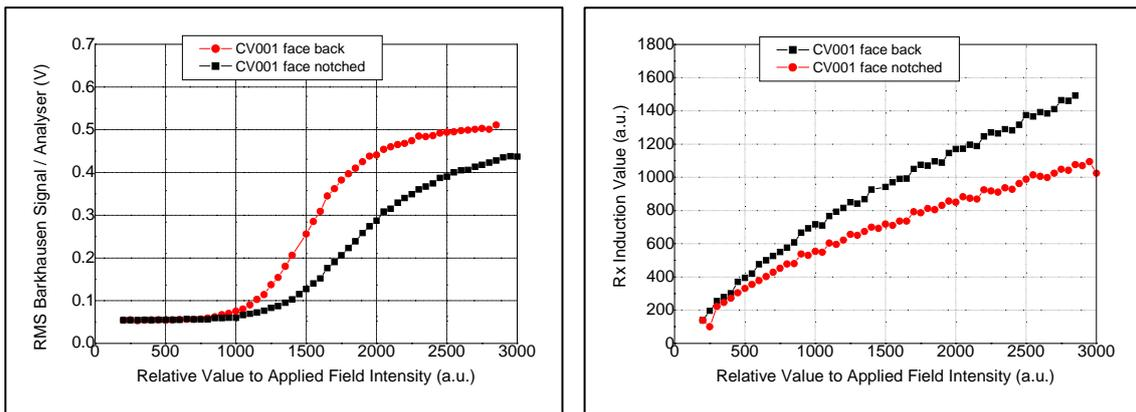
**Figure 3.** Barkhausen signal and RXI relative to induction value versus applied excitation intensity of irradiated specimens measured on two faces (100 Hz)
