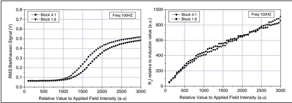
**Figure 2.** Barkhausen signal and RXI relative to induction value versus applied excitation compared on blocks 4.1 and 1.6
