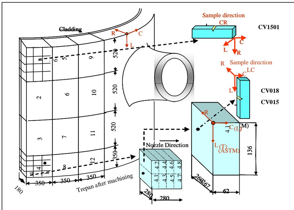
**Figure 1.** Pressure vessel and specimens cut diagram
