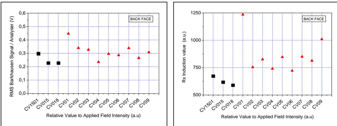
**Figure 7.** Barkhausen (left) and  $R_{X_I}$  (right) measurements on received (square) and irradiated (triangle) specimens (100Hz, 2000 constant level)
