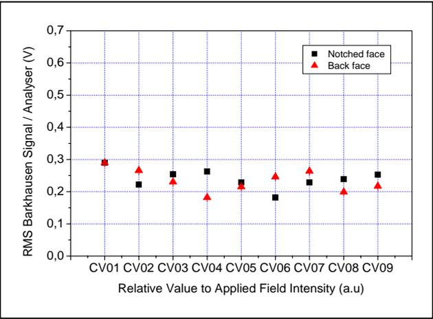
**Figure 5.** Comparison between two faces, back and notched of Barkhausen measurements on irradiated specimens (10Hz)
