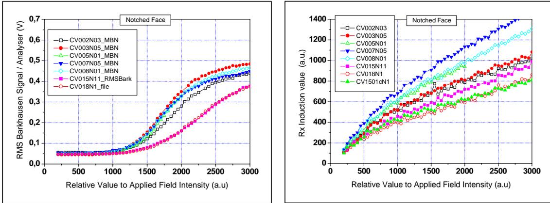
**Figure 6.** Barkhausen signal and  $R_{X_I}$  relative to induction value versus applied excitation intensity of irradiated and fresh specimens measured on notched face
