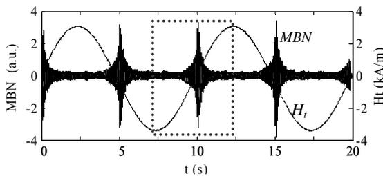
Figure 2 The MBN and  $H_t$  signals acquired during two complete hysteresis cycles applied to a low carbon steel sample.
