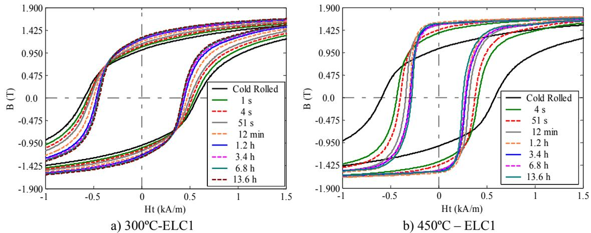
Figure 5 Evolution of the cold rolled ELC1 steel samples isothermally annealed and quenched at various stages.
