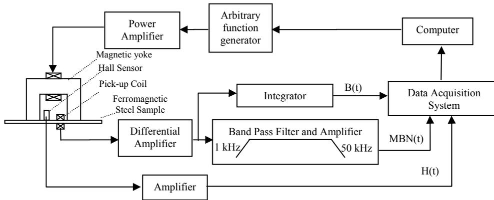
Figure 1 Schematic diagram of experimental setup for magnetic hysteresis loops and MBN measurements.
