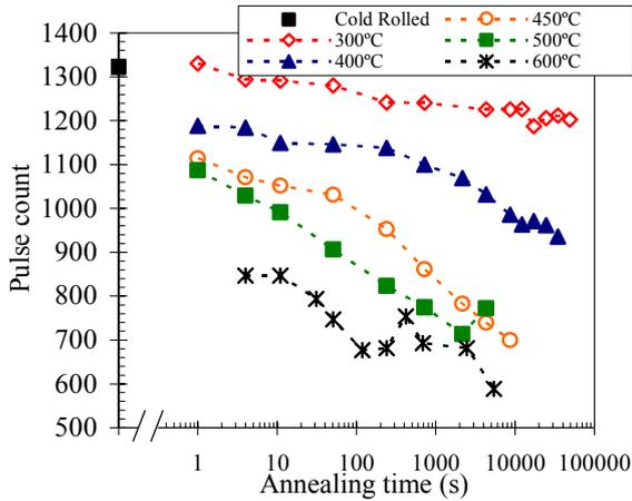
Figure 8 Total number of MBN pulses as a function of the annealing time.
