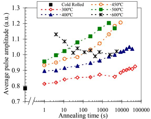
Figure 9 Average amplitude of MBN pulses as a function of the annealing time.
