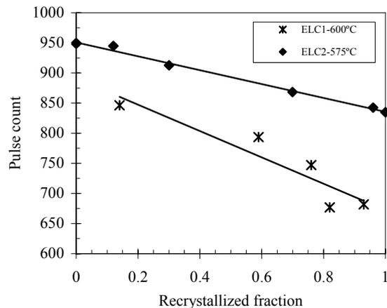
Figure 14 Correlation between the MBN number of pulses and the recrystallized fraction in ELC1 and ELC2.
