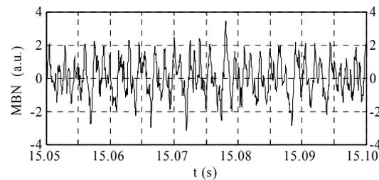
Figure 3 The MBN signal with an expanded time scale.
