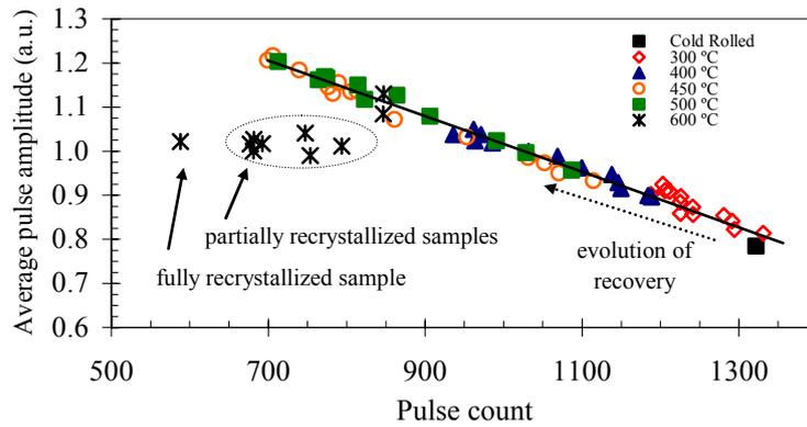
Figure 12 Correlation between the average amplitude and the total number of MBN pulses during recovery and recrystallization.
