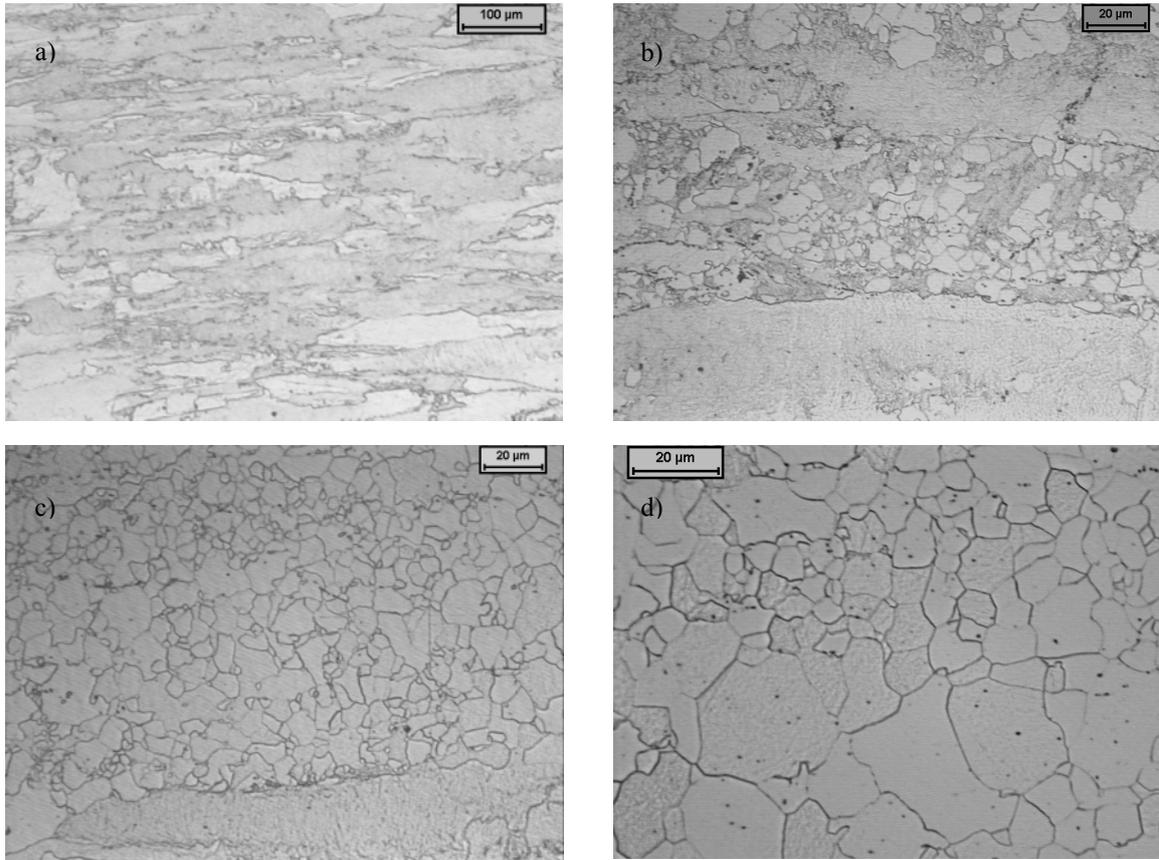
Figure 4 Optical micrographs showing the steel microstructure after different annealing treatments: a) 500 °C-4,8h; b) 600 °C-11s; c) 600 °C-240s; d) 600 °C-5400s.
