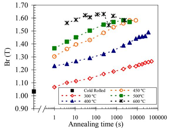
Figure 7 Evolution of the remanent induction with the annealing time.
