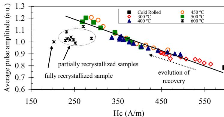
Figure 11 Correlation between the average amplitude of MBN pulses and the coercive field values during recovery and recrystallization.
