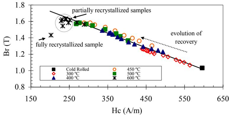
Figure 10 Correlation between remanent induction and coercive field values for the analysed temperatures during recovery and recrystallization.
