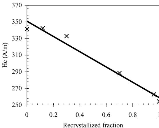
Figure 13 Correlation between the coercive field and the recrystallized fraction in ELC2.
