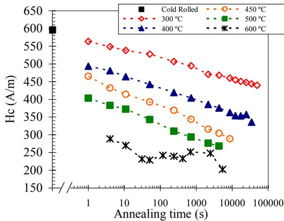
Figure 6 Evolution of the coercive field with the isothermal annealing time.
