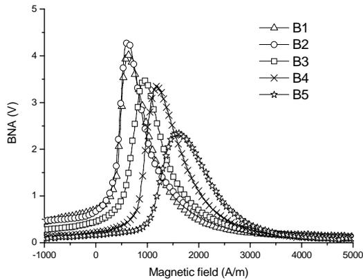
**Figure 3.** Barkhausen noise signals for different industrial DP steels
