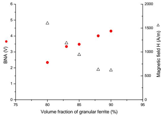
**Figure 4.** Barkhausen noise amplitude and peak position as a function of the proportion of granular ferrite for industrial DP steels
