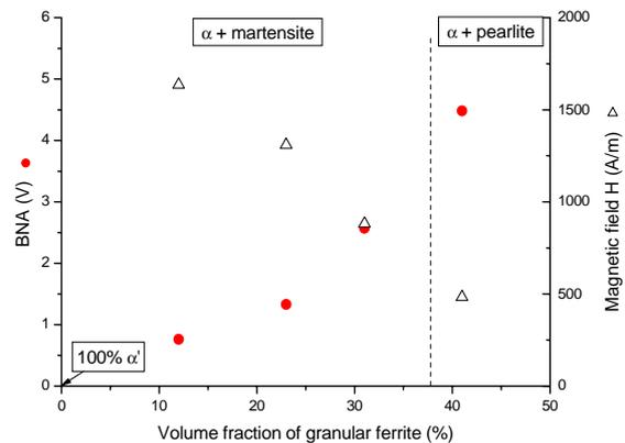
**Figure 2.** Barkhausen noise amplitude and peak position of ferrite as a function of its proportion for ferrite-martensite steels
