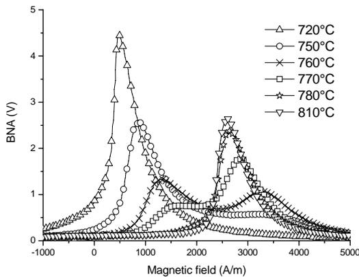
**Figure 1.** Barkhausen noise signals of ferrite-martensite steels as a function of the intercritical annealing temperature
