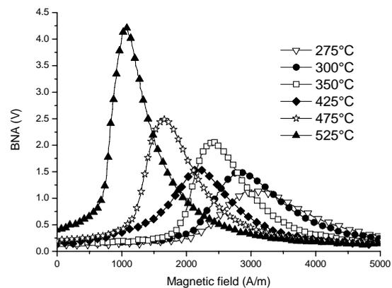
**Figure 5.** Barkhausen noise signals for isochronous treatments of 8 min
