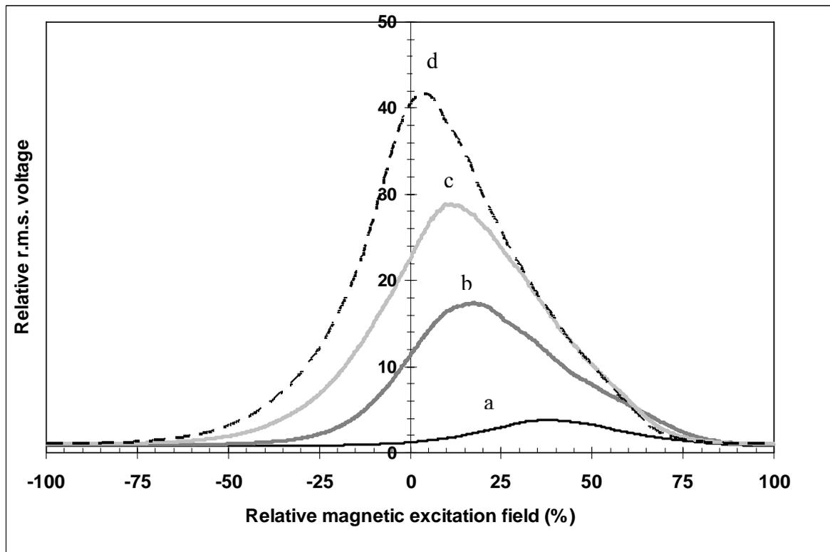
**Figure 3.** Relative r.m.s. Voltage versus Relative Magnetic Excitation Field Graphs for the Microstructures
