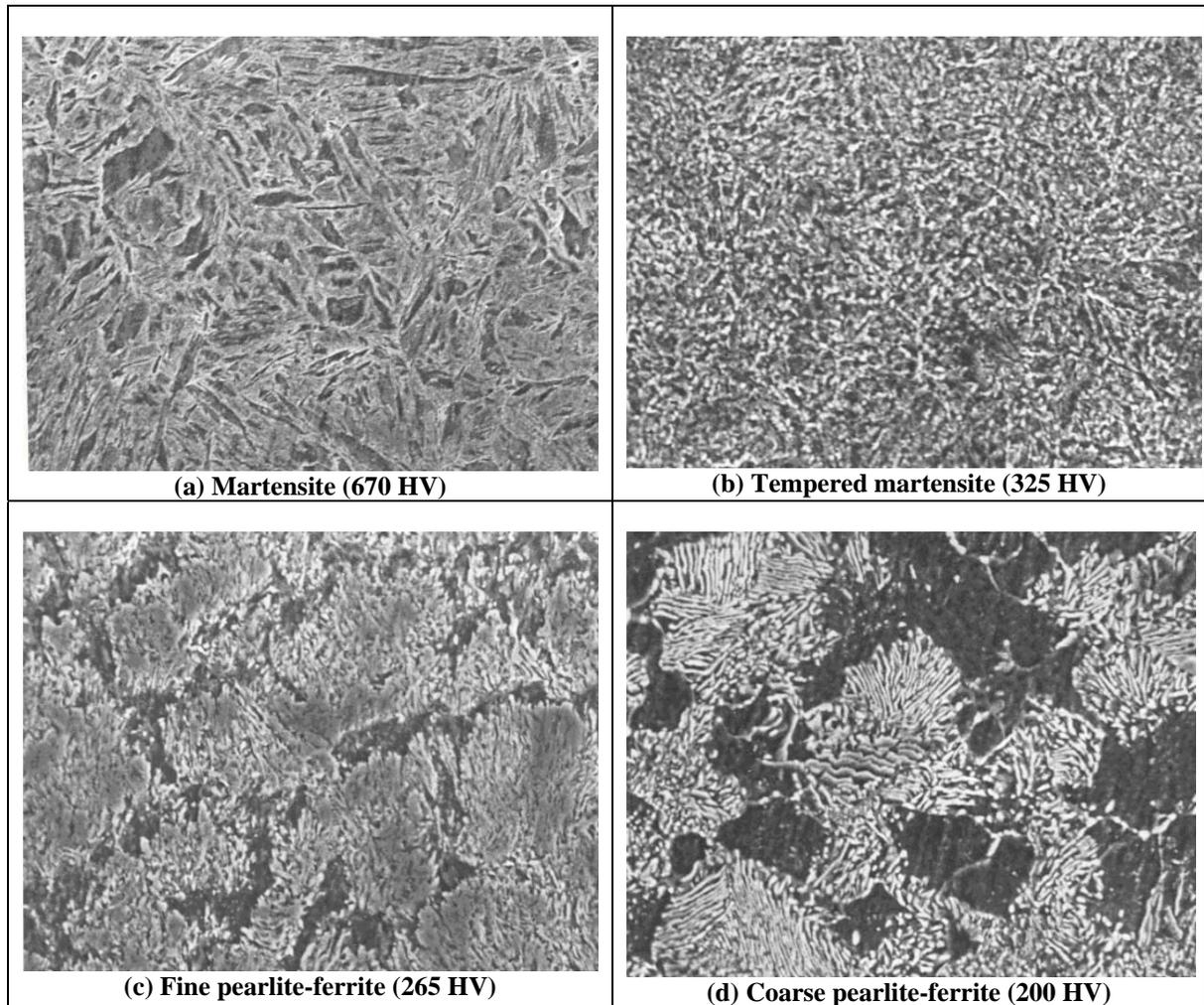
**Figure 1.** Representative Micrographs and Hardness of the Samples
