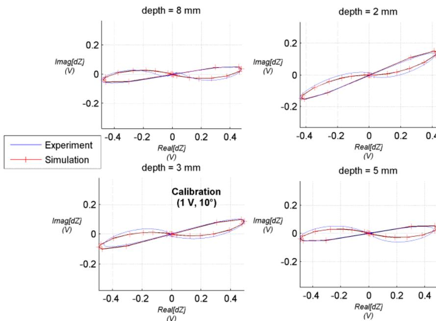
**Figure 3.** Experimental and computed signals obtained on the four holes tested with an off-centered probe
