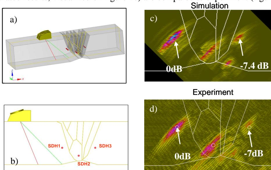
**Figure 1.** Simulation of the ultrasonic inspection of an austenitic weld; a and b) Simulated configuration; c) Simulated true Bscan; d) Experimental true Bscan
