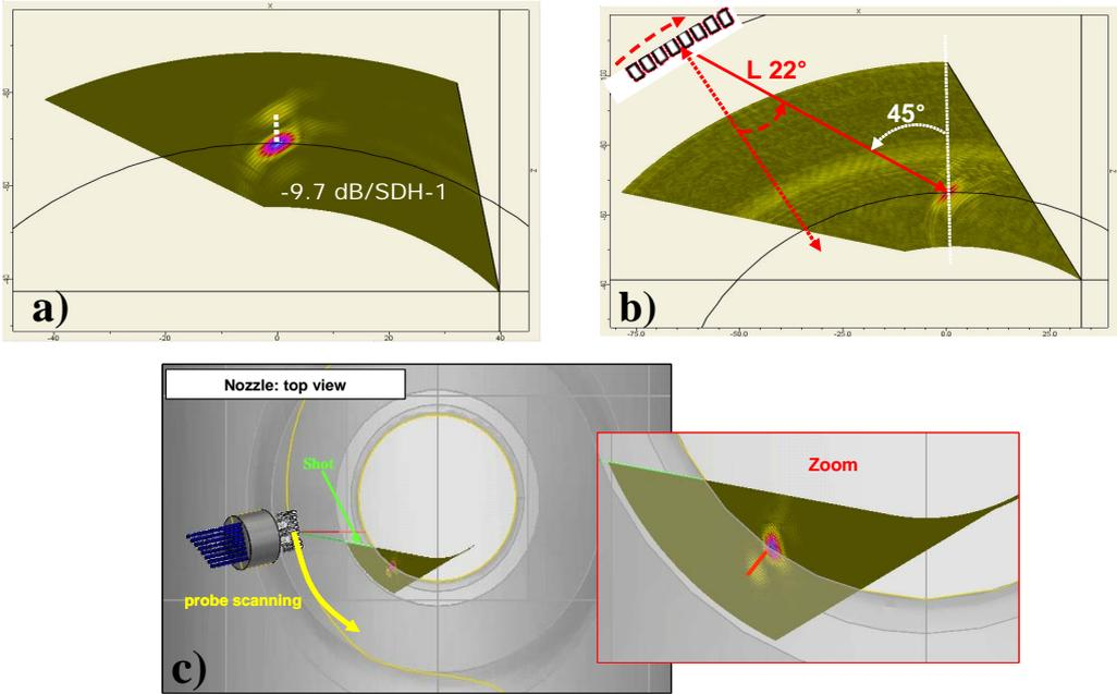
**Figure 5.** Simulation of the response of the notch of Figure 4; a) Simulated rectified Bscan ; b) Experiment; c) The simulated Bscan of a) visualized in the 3D view of CIVA
