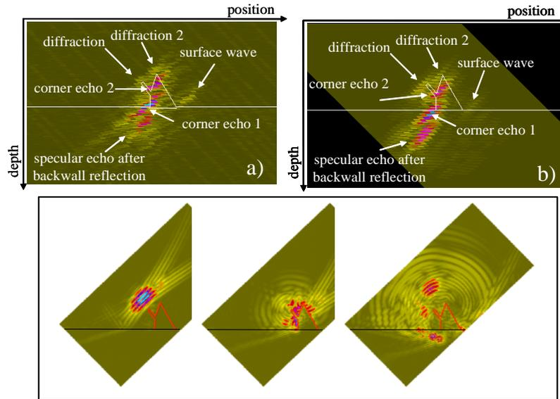
**Figure 8.** T45 Simulation of the inspection of a branched breaking crack; Experimental (a) and simulated (b) rectified Bscan images c) Successive snap-shots provided by the FEM computation
