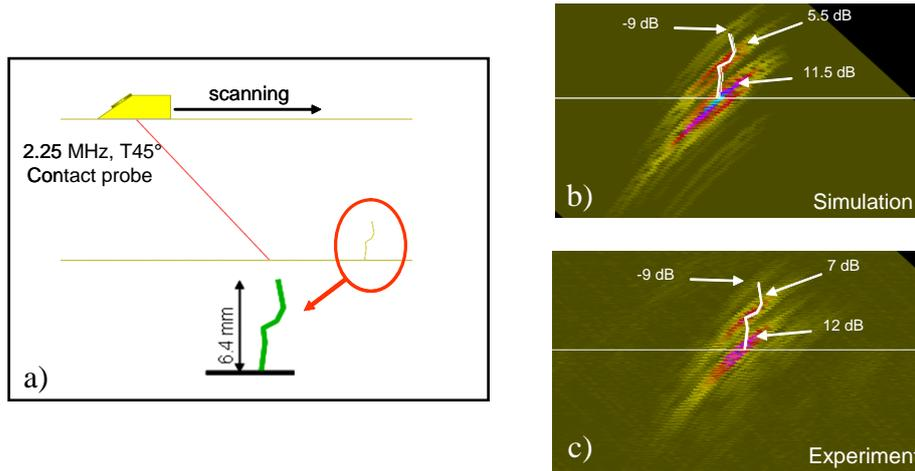
**Figure 7.** Simulation of the response of a multi-faceted defect; a) Simulated configuration, b) Simulated and c) experimental rectified Bscans.
