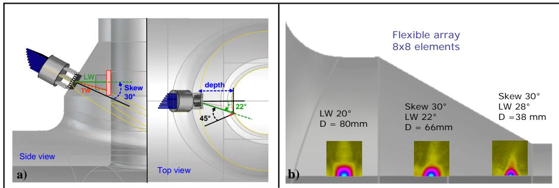
**Figure 4.** a) Visualization of one inspection configuration; b) Some results of field computations for different probe positions, the array being excited with optimized delay laws computed.
