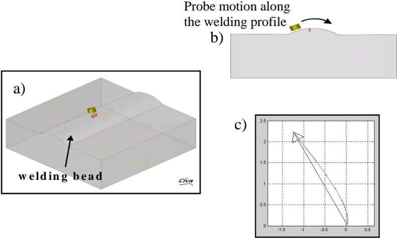
**Figure 6.** Welding inspection of a repaired Inconel area with a surface ridding probe; a) Configuration; b) extracted profile and c) simulated flaw response
