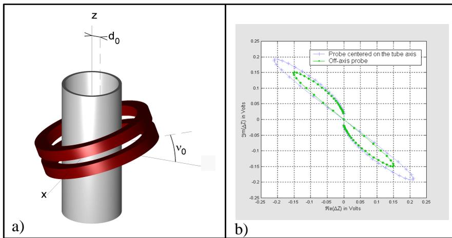
**Figure 2.** a) Tubing inspection configuration; b) Effect of a probe eccentricity: Computed signals arising from a longitudinal notch for both centered and off-centered probes
