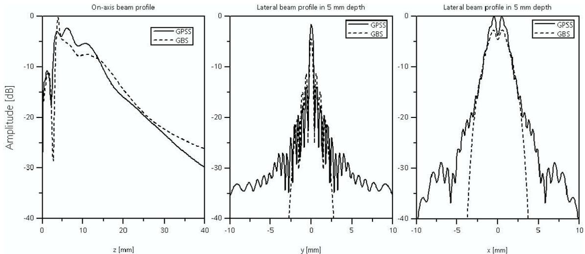
**Figure 4.** On-axis and lateral beam profiles in the focal plane (center) and perpendicular to it (right) in 5 mm depth of the titanium disc, calculated for Probe 2 using point source superposition (GPSS) and Gaussian beam superposition (5 beams).
