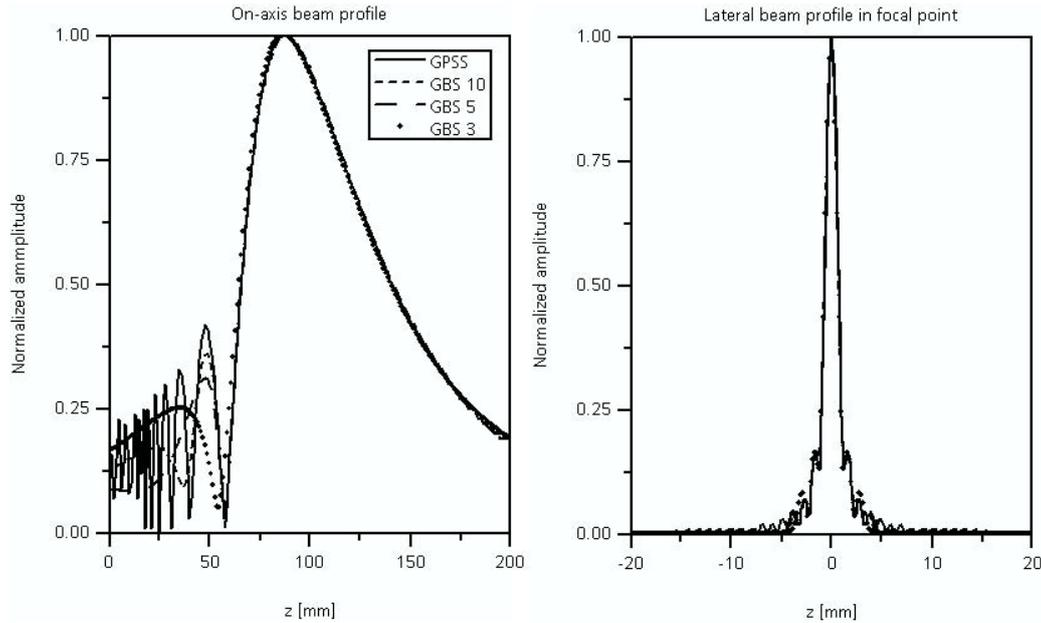
**Figure 2.** On-axis and lateral beam profile in the focal point for Probe 1 (in water), calculated using point source superposition (GPSS) and Gaussian beam superposition for a three-, five- and ten-term solution.
