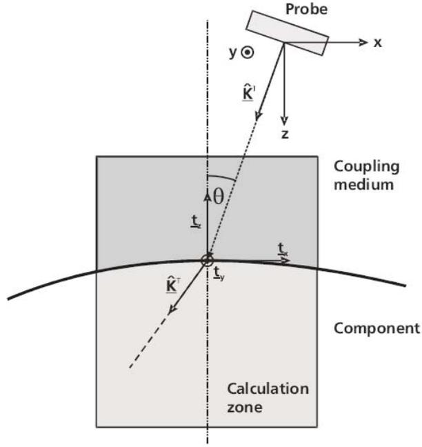
**Figure 1.** Principal set-up of probe, component and the coordinate system in considering the transmission problem in view of immersion testing.
