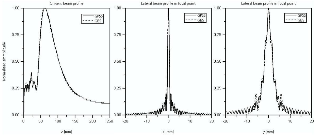
**Figure 3.** On-axis and lateral beam profiles in the focal plane (center) and perpendicular to it (right) in the focal distance for Probe 2 (in water), calculated using point source superposition (GPSS) and Gaussian beam superposition (5 beams).
