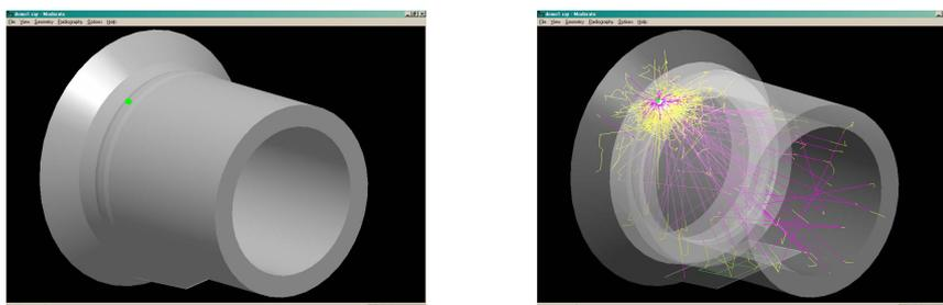
**Figure 1:** one MODERATO configuration used in a RT procedure qualification program (left) and illustration of some photon trajectories inside the pipe, as calculated by MODERATO's Monte-Carlo algorithm.
