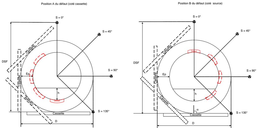
**Figure 3:** Source - Defect - Film orientations. A (left): defect on film side, B (right): defect on source side.
