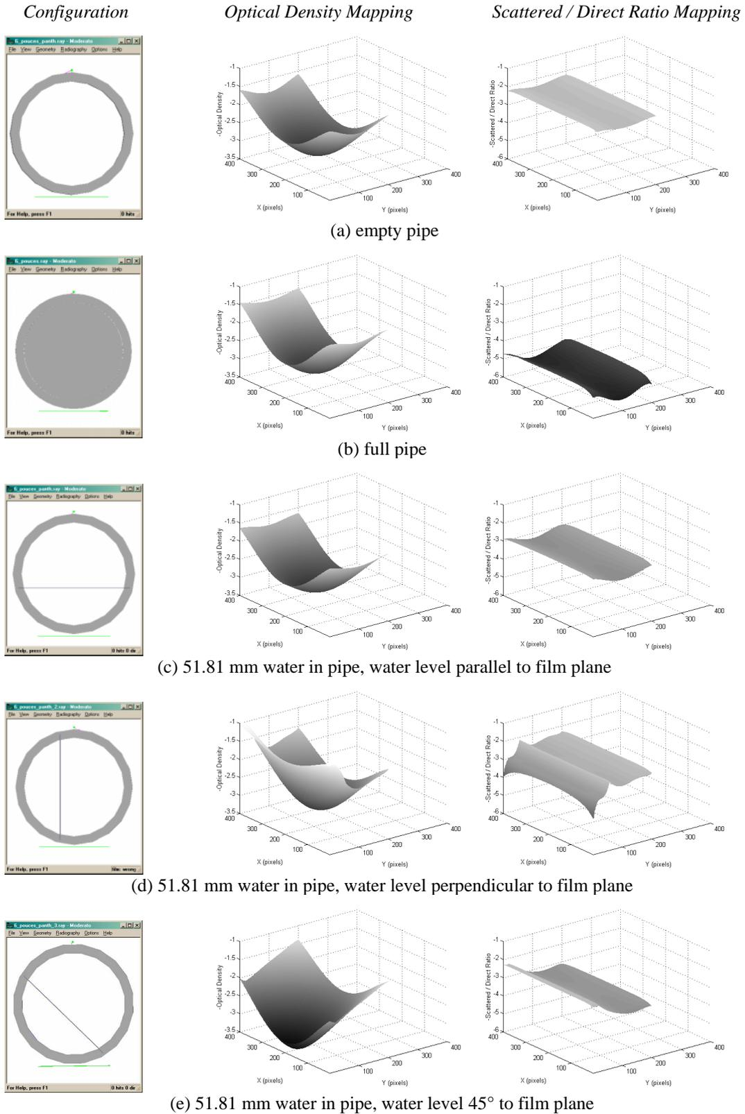
**Figure 4:** Configuration (left), Optical Density Mapping (centre) and Scattered / Direct Ratio Mapping (right) for the five configuration series. The vertical scales are oriented downwards in order to have a better correspondence between optical density and graph's gray-scale.
