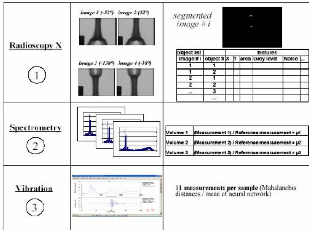
Figure 3 : Data processing for the three methods.
