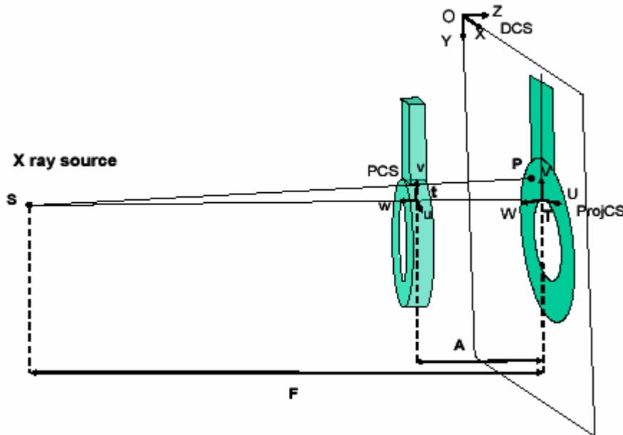
Figure 6 : Representation of the radioscopic bench, with three coordinate systems.
