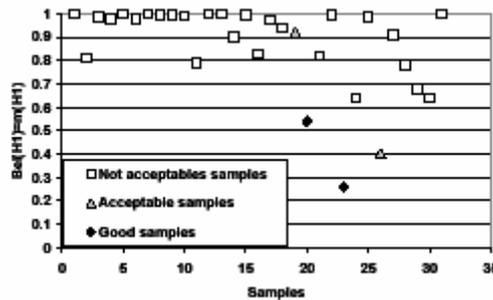
Figure 14 : Plot of the 31 samples having a belief in the  $H_1$  hypothesis , labeled with the end user acceptability
