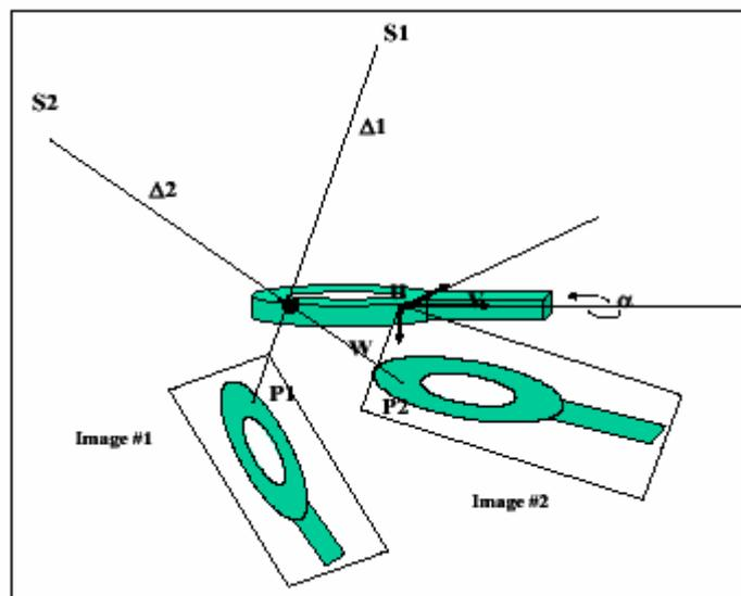
Figure 7 : Representation of the two lines  $\Delta (S,P)$  for a sample, depending on the radiographic orientations.
