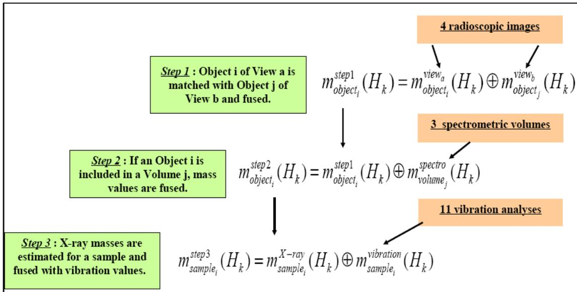
Figure 5 : Schematic diagram of the 3 fusion steps for one sample. The symbol  $\oplus$  refers to the Dempster rule of combination (relation (1)).
