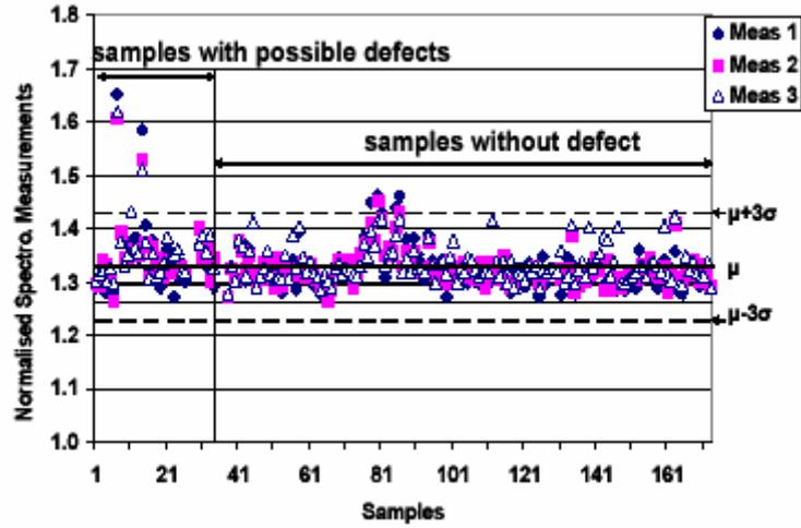
Figure 10 : Three spectrometric measurements done for each sample, after the normalisation with reference thickness values.
