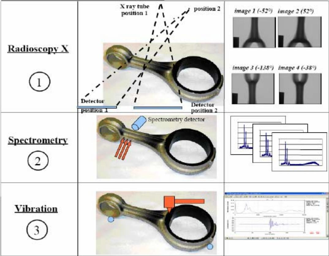
Figure 2 : The three acquisition steps and the corresponding output data.
