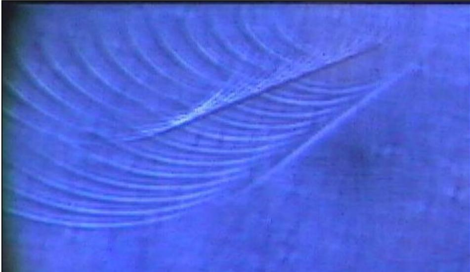
Figure 8 PhotoElastic Image Showing Wave Front Components
