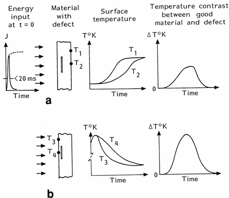
Fig 1. Schematic representation of the transient thermography method (a) through transmission (double sided); (b) reflection (single sided). (after [1,3])
