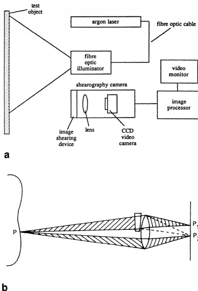
Fig 2. (a) Shearography equipment (after [1,13]); (b) schematic representation of shearing process (after [1]).
