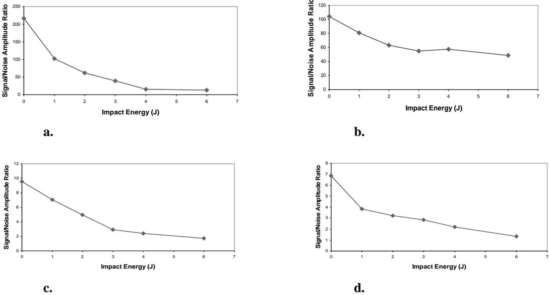
Figure 6. Curves showing the signal-to-noise amplitude ratio as a function of the impact energy: a. Surface mounted SMARTape sensor; b. Embedded SMARTape sensor; c. Embedded locally stripped SMARTape sensor; d. Embedded bare optical fibre sensor.
