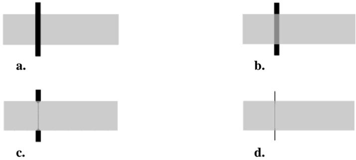
Figure 5. Different fibre integration methods: a. Surface mounted SMARTape sensor; b. Embedded SMARTape sensor; c. Embedded locally stripped SMARTape sensor; d. Embedded bare optical fibre sensor.
