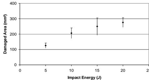
Figure 10. Curve showing the damaged areas calculated from ultrasonic C-scan images for quasi-isotropic carbon/epoxy samples impacted at different energy levels.
