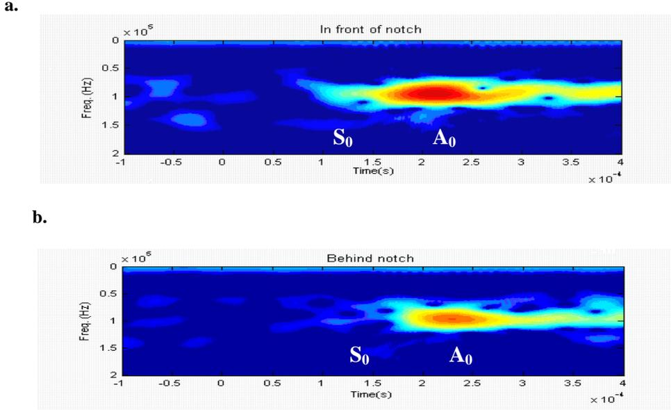
Figure 8. Time-frequency spectrum of the signals received in a notched aluminium plate: a. Signal received in front of the notch; b. Signal received behind the notch.
