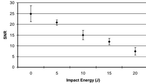
Figure 9. Curve showing the RMS-based SNR for quasi-isotropic carbon/epoxy samples impacted at different energy levels.
