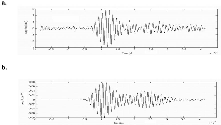
Figure 4. Signal recorded in a carbon/epoxy specimen after excitation of a 5 cycle sine burst at 100 kHz: a. Signal recorded by a SMARTape sensor; b. Signal recorded by a conventional piezo transducer.
