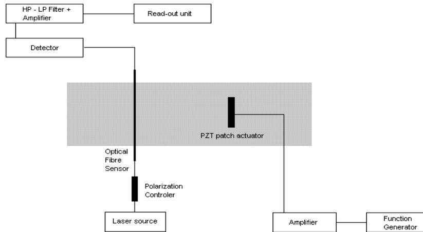
Figure 1. Single mode optical fibre sensor in a polarimetric setup for the detection of impact damage
