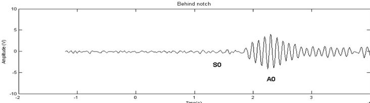
Figure 7. Signals received in a notched aluminium plate: a. Signal received in front of the notch; b. Signal received behind the notch.
