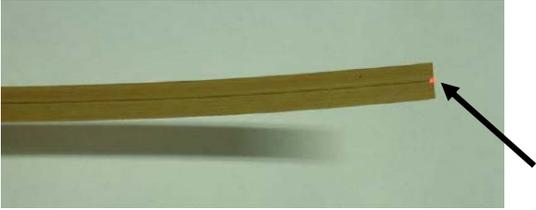
Figure 2. Picture of the SMARTape optical fibre sensor with visible light. [15]
