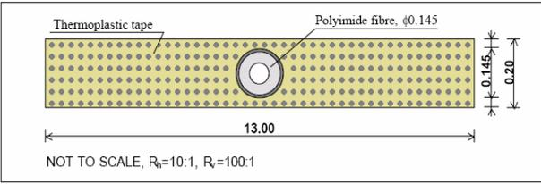
Figure 3. Cross-section of the SMARTape optical fibre sensor. [15]
