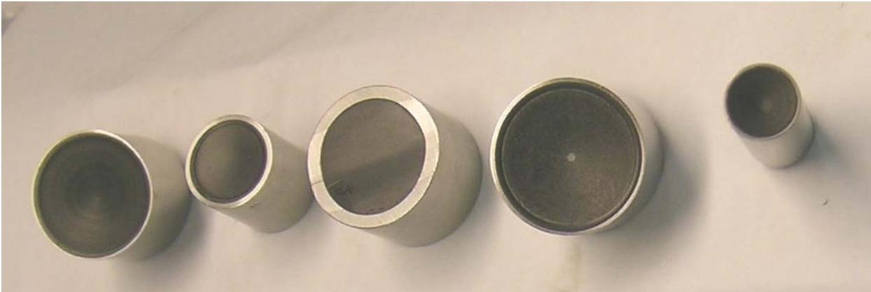
Figure 2. Transducers with acoustic logarithmic lenses.
