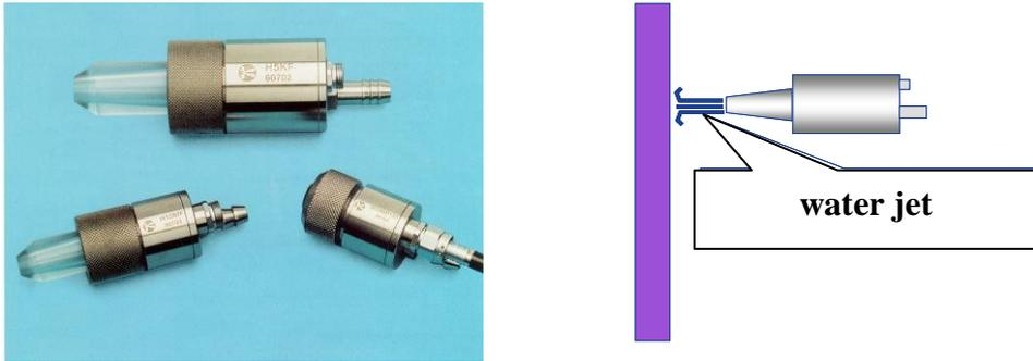
Figure 9 Squirter probe and principle of coupling via a waterjet
