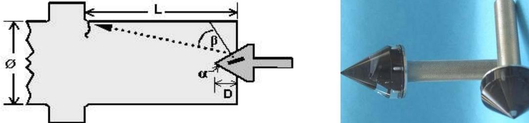
**Figure 14** Cone Probe for Testing of railway Wheelset Axles for circumferential cracks from the center hole
