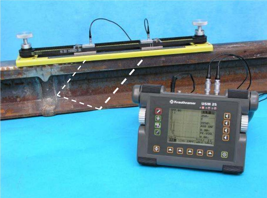
**Figure 13** Rail Tandem Scanner STH2
