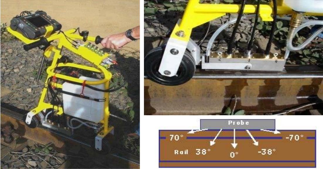
**Figure 12** Rail Test Trolley SPG2 with Special Probe and Sound Directions
