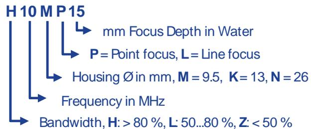
**Figure 8** Nomenclature of the Immersion Probes
