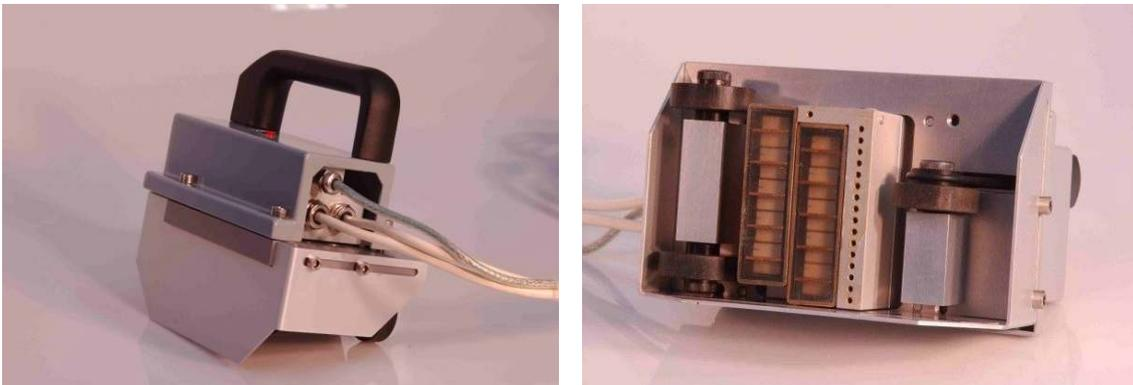
**Figure 20** Manual Scanning Device. The right picture shows the scanning device from the bottom.
