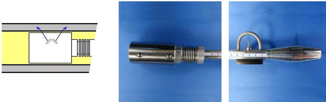
**Figure 17** Double Angle Beam Probe for the detection of transverse flaws in hollow axles
