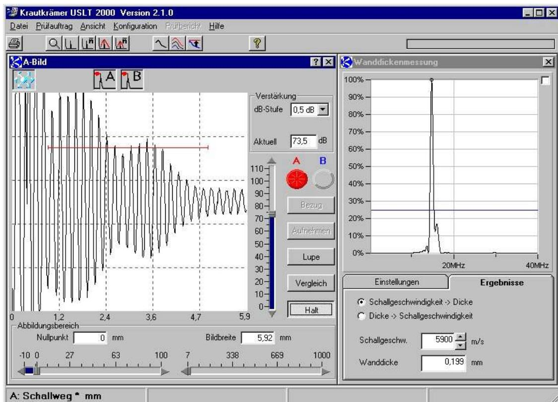
**Figure 2** Thickness measurement by evaluation of the resonance signal of a 0,2mm steel plate – Result: 0.199 mm
