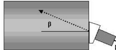
**Figure 15** Attachable wedge for testing from the axles front face
