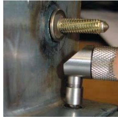
**Figure 4** Spot Weld Probe G 20 MN 3,2 X B2
