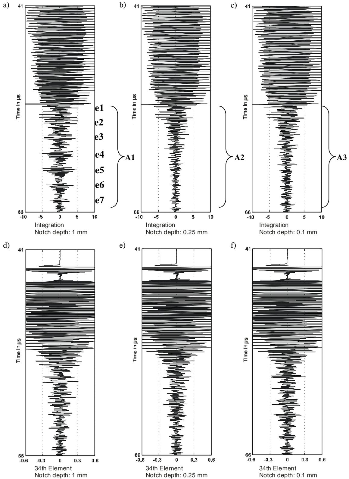
Figure 5: A-scans obtained by EFIT simulations with different notch depths. The averaged A-scans shown in a), b), and c) are obtained by averaging the A-scans in their respective parallel B-scans. The A-scans shown in d), e), and f) are the A-scans obtained by the 34<sup>th</sup> element of the 64 element phased array transducer with different notch depths indicated under the A-scans.
