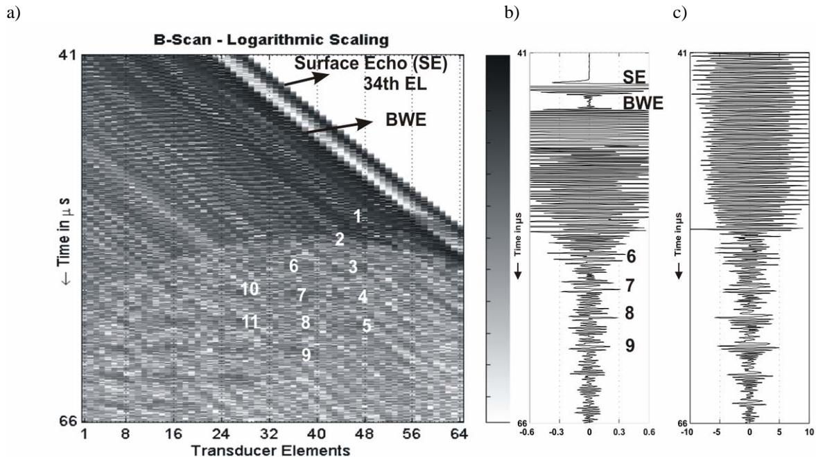
Figure 4: 2-D EFIT results for a steel slab with a surface breaking notch of 1 mm of depth and 0.3 mm of width immersed in water and a 64 element phased array transducer with a carrier frequency of  $f_c = 6$  MHz: a) parallel B-scan with linear scaling and echo interpretation, b) A-scan obtained by the 45<sup>th</sup> element, c) A-scan obtained by averaging the A-scans of the parallel B-scan given in a)
