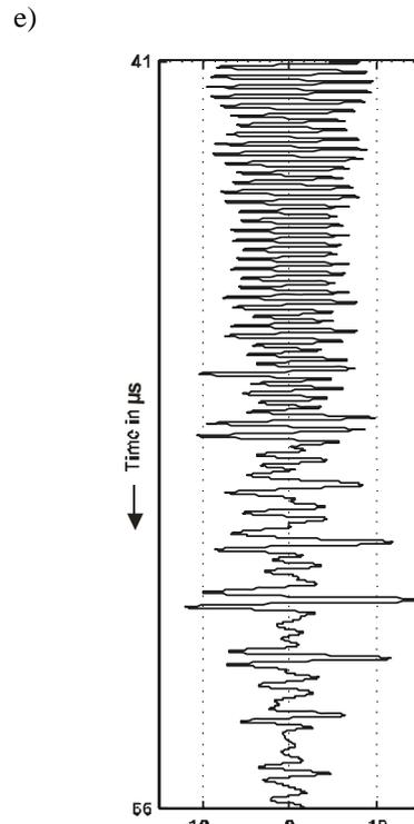
Averaged EFIT A-scan computed from the parallel B-scan,  $f_c=2$  MHz
