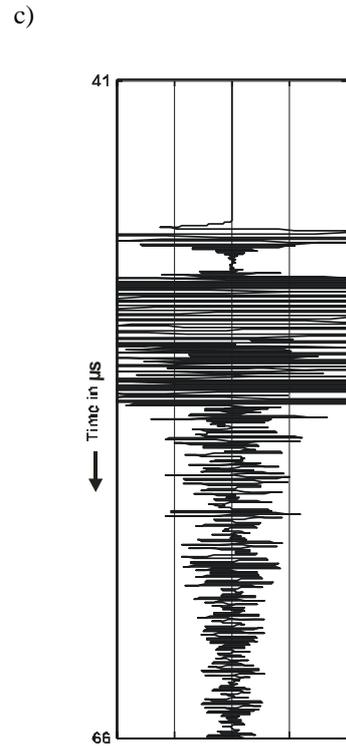
EFIT A-scan at the 45<sup>th</sup> element,  $f_c=6$  MHz
