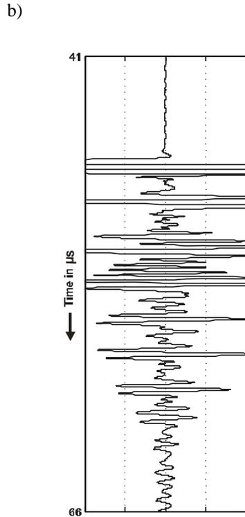
EFIT A-scan at the 45<sup>th</sup> element,  $f_c=2$  MHz
