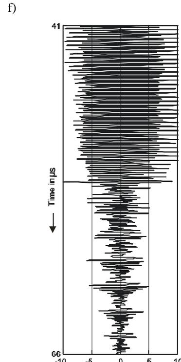
Averaged EFIT A-scan computed from the parallel B-scan,  $f_c=6$  MHz
