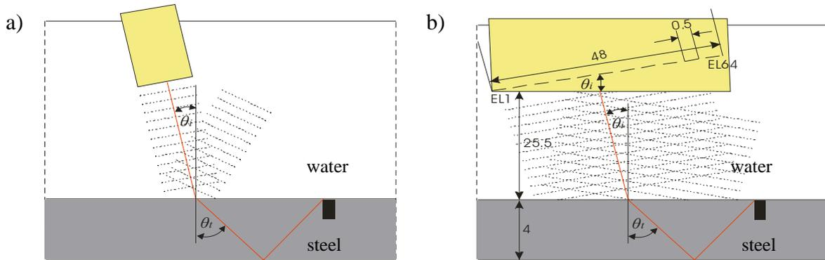
**Figure 1:** NDT of a pipeline: a) conventional ultrasonic probe, b) phased array transducer for the application of the real-time B-scan technique [8]
