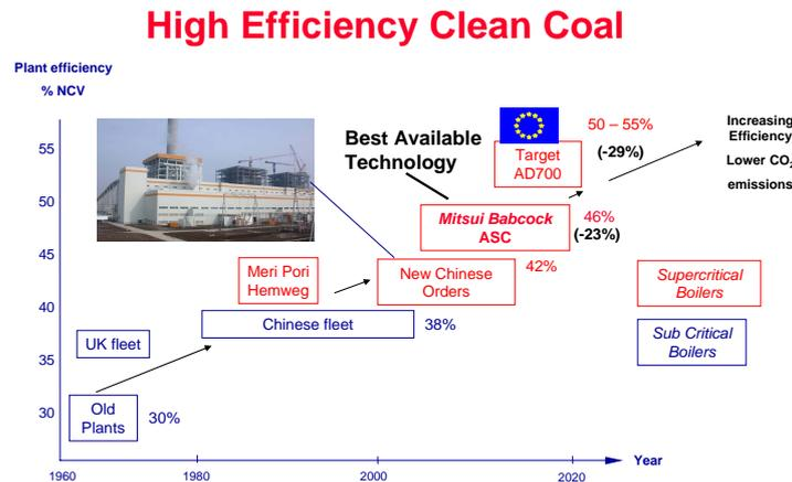
Figure 4 : Progressive improvement in efficiency and reduction of CO<sub>2</sub> emissions for coal-fired power plant
