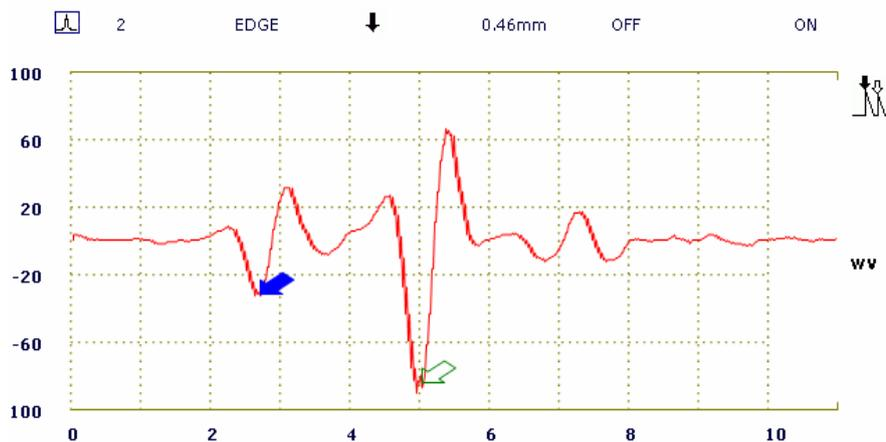
**Figure 3.** Typical internal oxide measurement with Panametrics-NDT EPOCH 4 flaw detector and 20 MHz normal incidence delay line transducer. Scale thickness is 0.46 mm.
