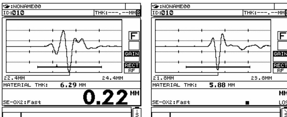
**Figure 2.** Shear wave measurement of thin oxide (left) and single peak tube wall waveform associated with disbonded oxide or oxide not present (right).
