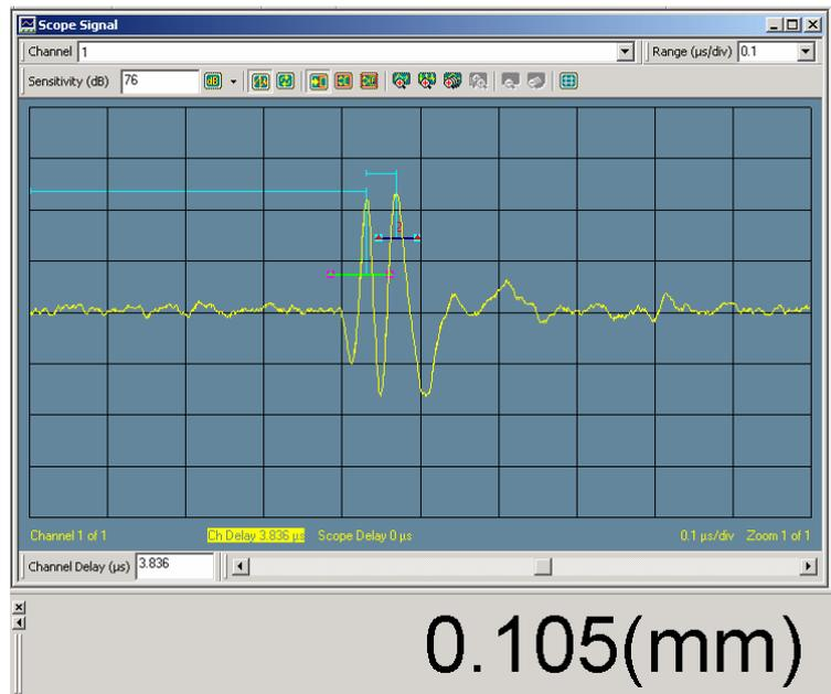
**Figure 4.** Measurement of 0.105 mm oxide scale with 50 MHz delay line transducer.
