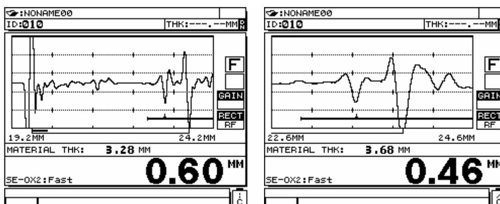
**Figure 1.** Typical internal oxide measurements with Panametrics-NDT Model 37DL PLUS thickness gage using 20 MHz transducer. Waveform on right has been zoomed to show details of oxide echo shape.
