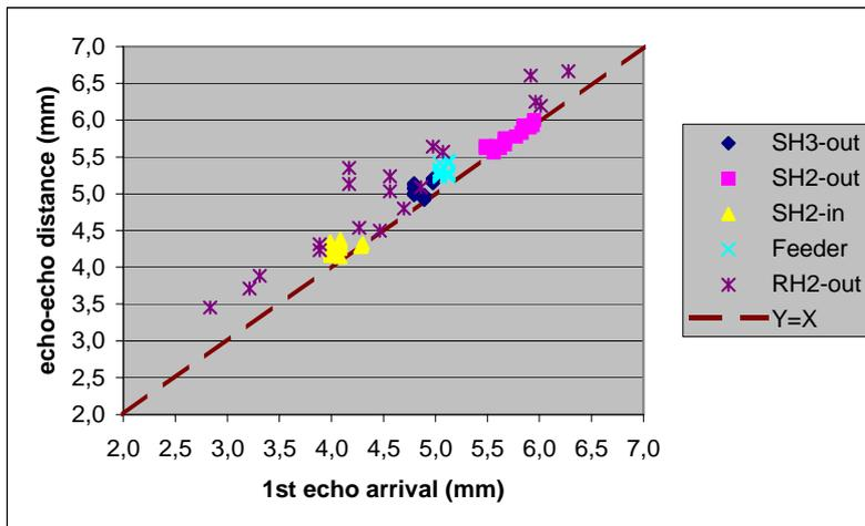
**Fig.3** – EMAT thickness data on oxidised boiler tubes: echo-echo distance generally exceeds 1<sup>st</sup> echo arrival.
