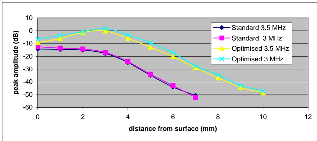
**Fig.7** - Comparison of the signal amplitude from two EMAT probes of different design on an aged tube.
