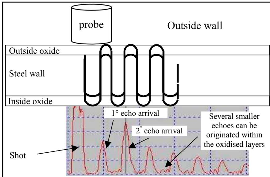
Fig.4 – Schematic of the ultrasonic pulse in a layered material with oxide on inside and outside walls
