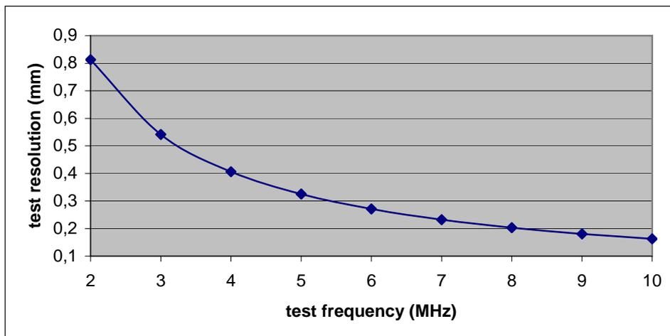
**Fig.8** - A EMAT system operating at up to 10 MHz would evaluate oxidised layers lower than 0.1 mm.
