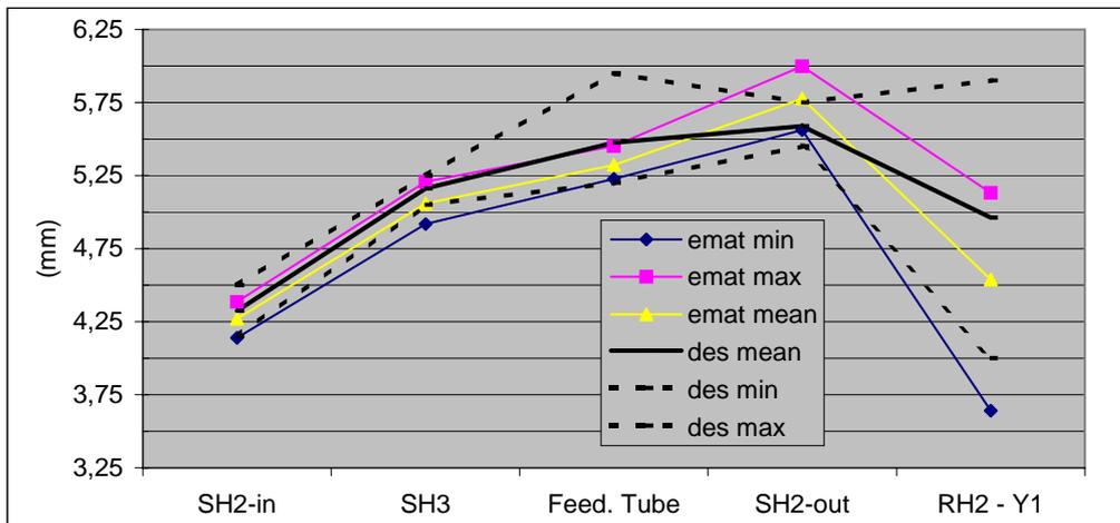
Fig.5 - Comparison between EMAT (echo-echo distance) and actual tube thickness (outer oxide included).
