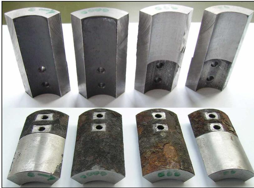
**Fig.6** - Tube samples machined for calibration on different wall conditions.
