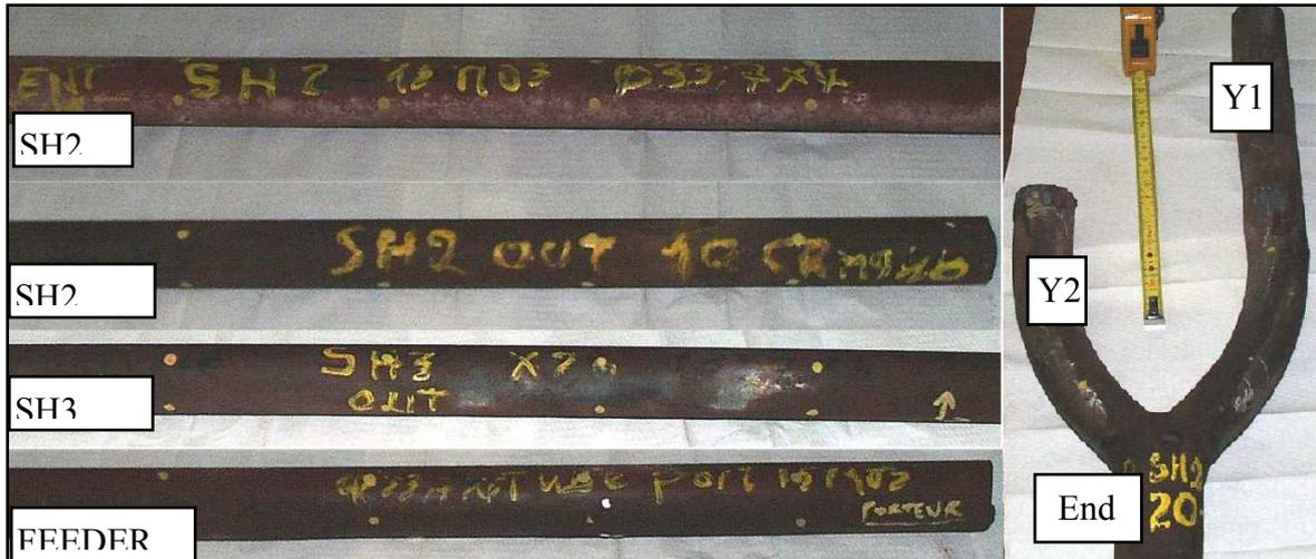
**Fig.1** – Aged boiler tubes considered for evaluation of EMAT thickness gauging from oxidised surfaces.
