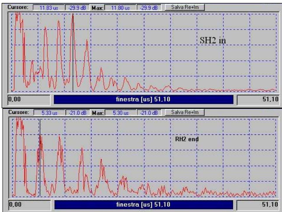
**Fig.2** - EMAT test. Upper: tube SH2-in, oxidised without scale. Lower RH2-end, a scaled and oxidised tube.
