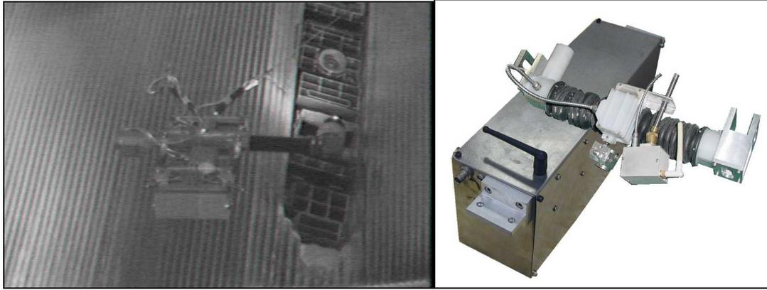
**Fig.9** - A waterwall climbing robot for visual inspections (left) and the EMAT kit for thickness gauging.
