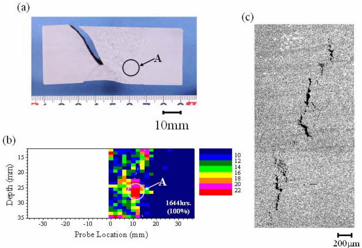
**Figure 5.** (a) A cross sectional picture of the ruptured specimen, (b) ultrasonic test result after rupturing and (c) a magnified picture at region A
