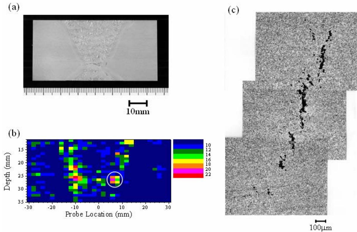
**Figure 3.** The result for the aborted specimen (650°C, 58.8MPa, 3449hrs., 60.1%) (a) a cross sectional picture, (b) an ultrasonic test result and (c) a magnified picture of the circled region
