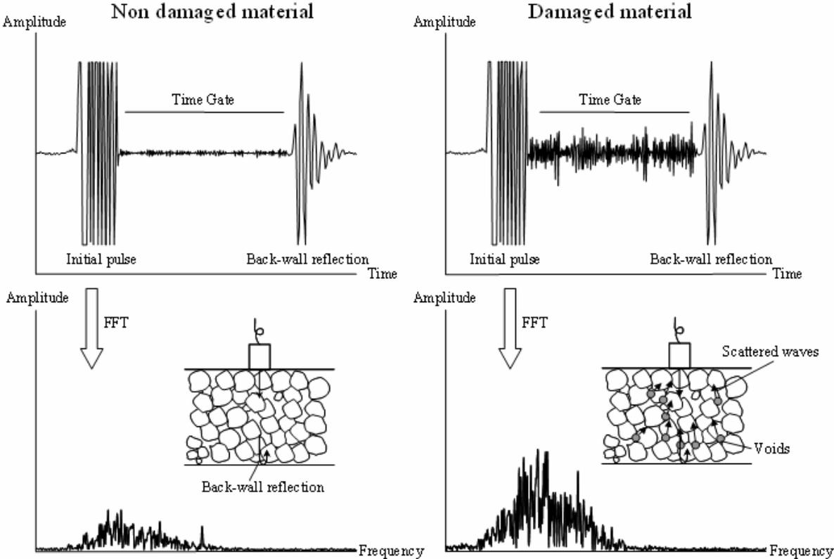
**Figure 1.** Schematic image of the scattering inside materials
