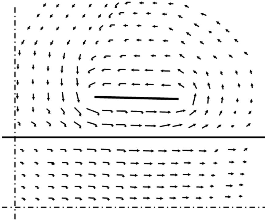
Fig. 9: Calculated magnetic field in the equidistant mesh points of Fig. 7. ( $F=1$ ,  $\mu=1$ )
