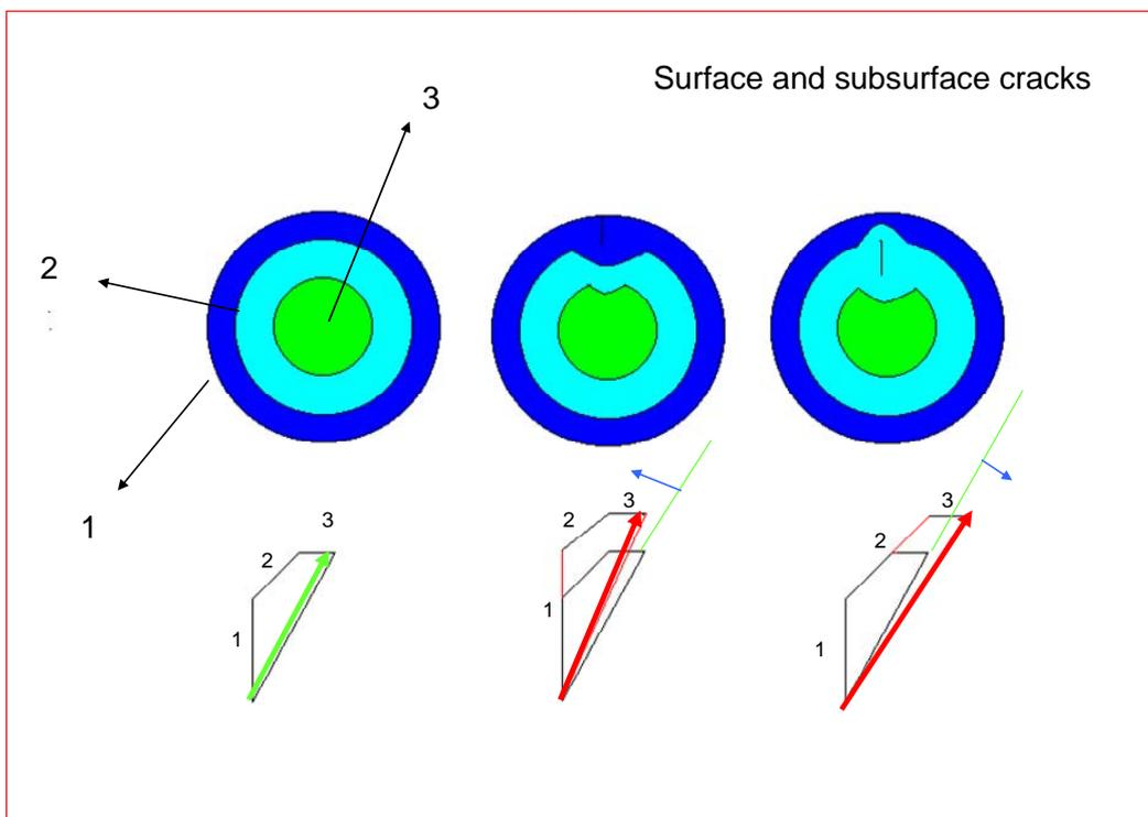
Fig. 4: Cross-section of a metal bar with a radial crack and without a crack. Surface cracks rotate the signal in the opposite direction than do the subsurface cracks.
