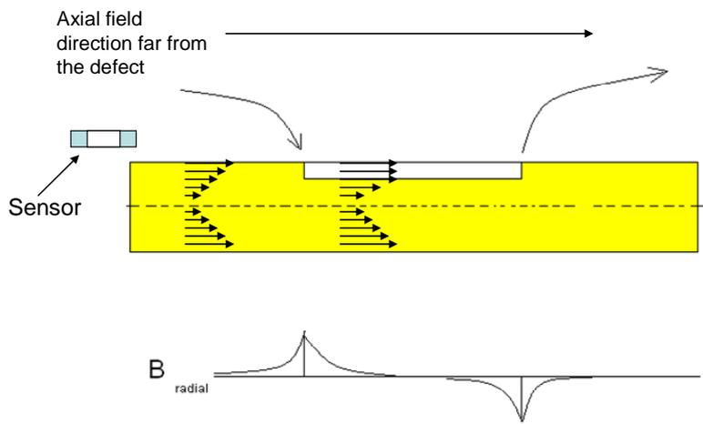
Fig. 6: Sensor for registration of the radial field.
