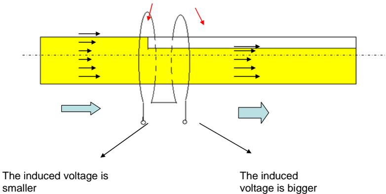
Fig.5: Differential arrangement of coils.
