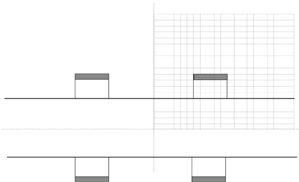
Fig. 8: Mesh of points where the magnetic field is calculated.
