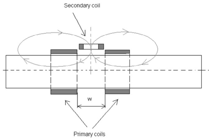
Fig. 7: Two parts of primary coils and the secondary coil measuring radial field.
