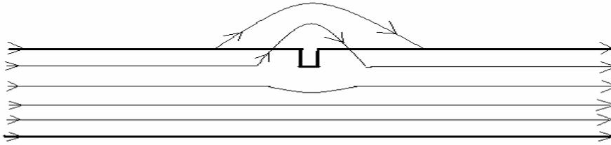
Fig.1: Magnetic leakage fields in the vicinity of a surface crack in the cross-section of a ferromagnetic plate.
