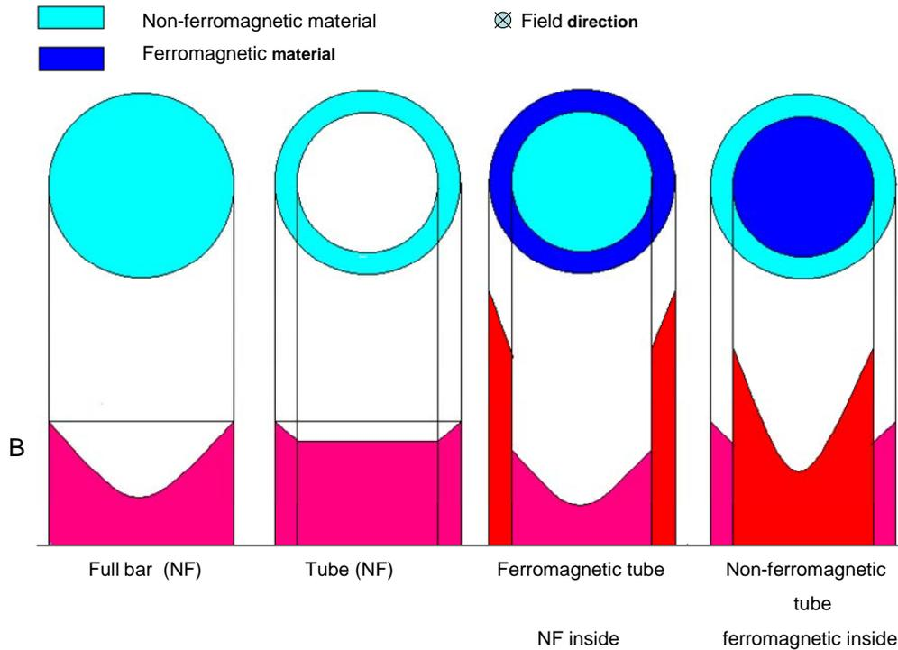
Fig. 2: Magnetic field density in circular cross-sections of different materials in longitudinal homogenous magnetic A.C. field.
