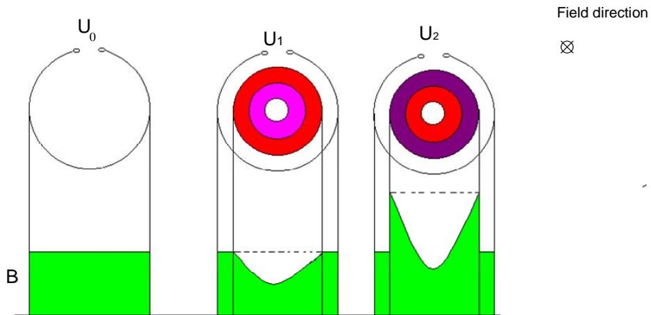
Fig. 3: The induced voltage is proportional to the encircled magnetic flux in free space ( $U_0$ ), in a non-ferromagnetic ( $U_1$ ) and in a ferromagnetic ( $U_2$ ) cross-section.
