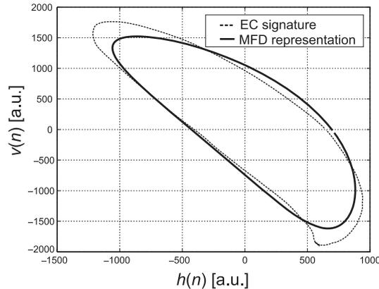
Fig. 4. EC signature representation via Modified Fourier descriptors using the first two descriptor orders
