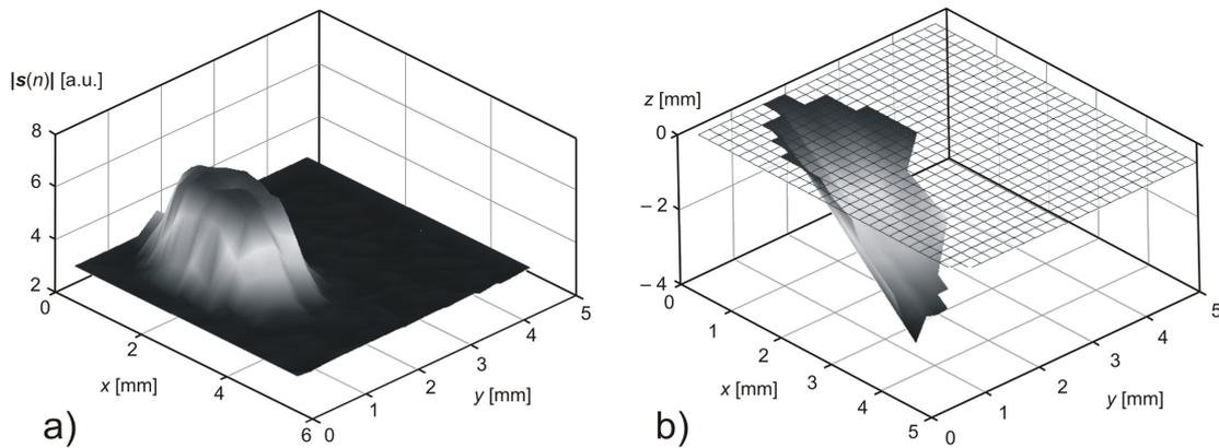
Fig. 5. Visualization of a flaw based on Fourier transformation
