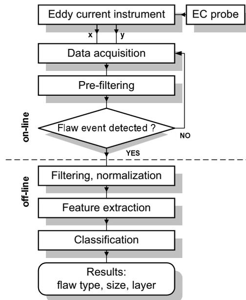
Fig. 1. Block diagram of EC inspection system with automated analysis of the EC signal
