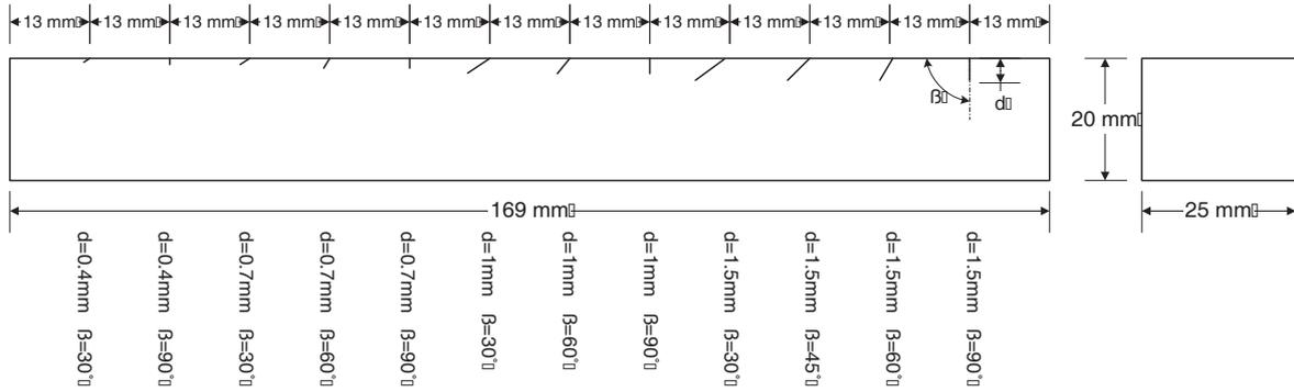
Fig. 6. Tested sample with machined notches (width 0.3 mm, length 25 mm, depth  $d$ , angle  $\beta$ )
