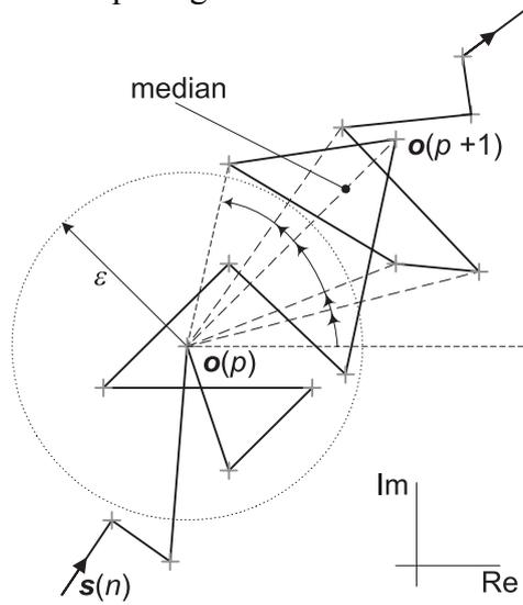
Fig. 3. Median signature tracking algorithm [2]:  $s(n)$  is the input noisy signature,  $o(p)$  is the output sample from the previous tracking step, and this sample also serves as the origin for the evaluation of sample angles,  $o(p+1)$  is the output sample selected via the median of the sample angles, and  $\varepsilon$  is the size of the circular neighborhood.
