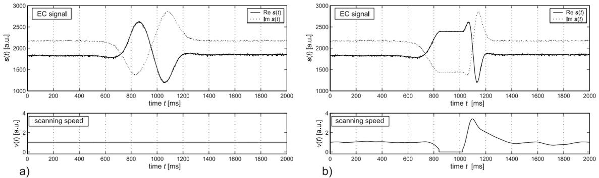
Fig. 2. Signal from EC probe for: a – motorized positioning, b – manual scanning by human operator. The same instrument and setup were used. The flaw width on surface was 0.3 mm.
