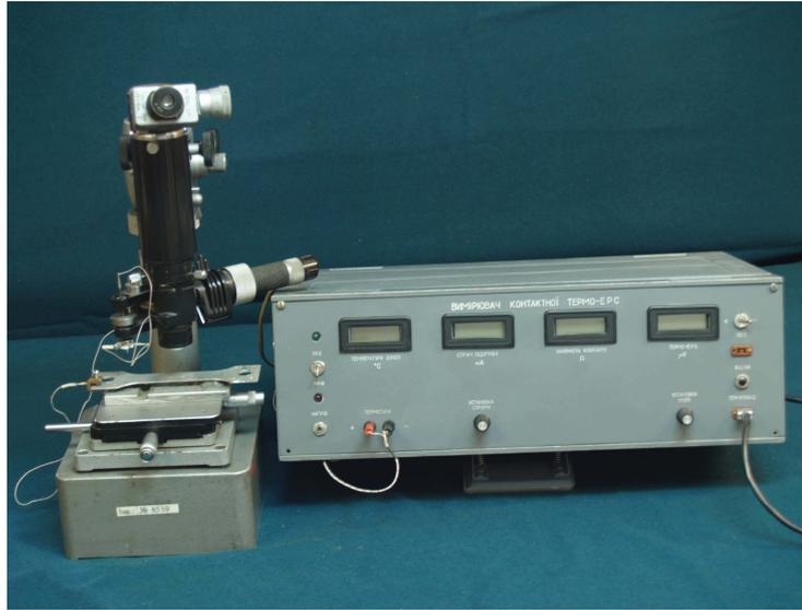
Figure 3. The experimental device for local TEP measurement - «Contact-1».
