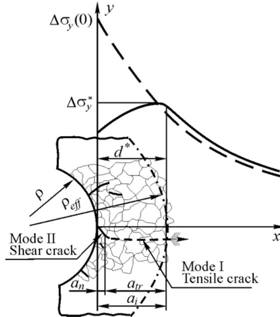
Figure 1. Schemes of FPZ formation and stress distribution at the tip notch (a) and growth of small fatigue cracks in this zone (b).
