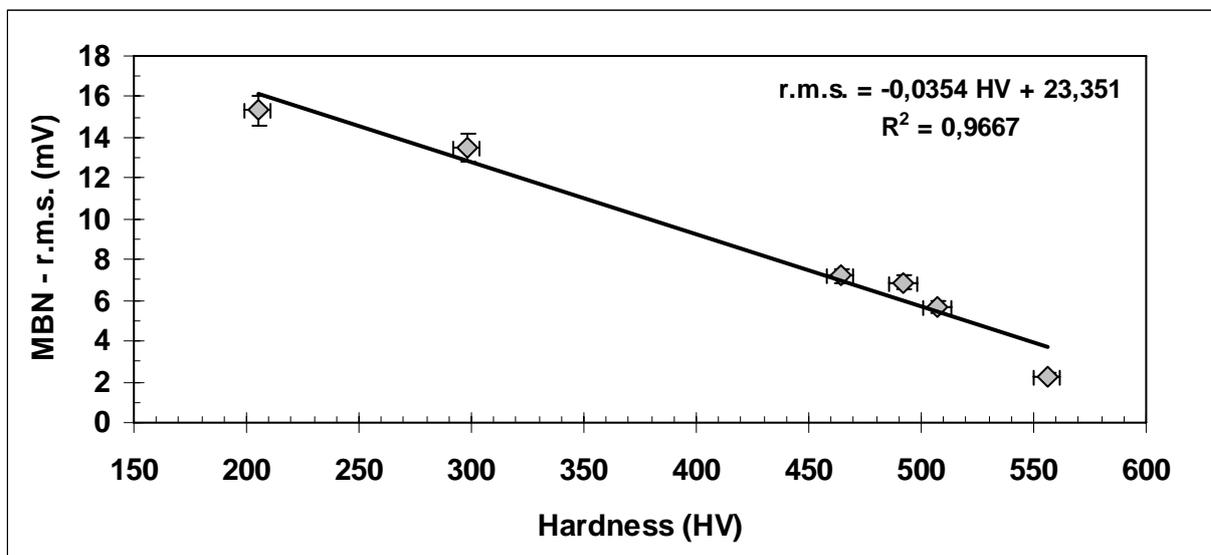
Figure 3. Correlation of MBN-r.m.s. Values with Hardness
