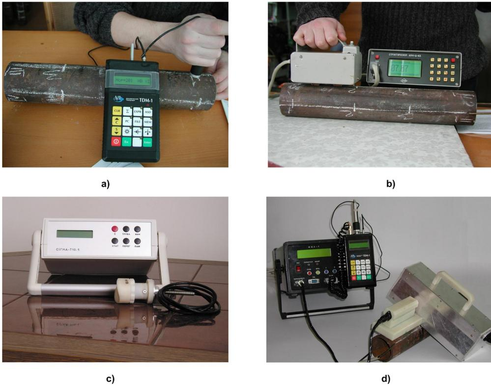
a) – hardness meter TDM-1; b) – coercive force meter KRM-CK;
