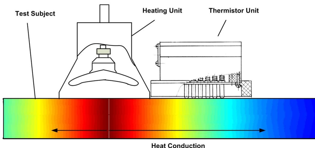
**Fig.3.** Positional relationship of heating and thermistor unit on the surface of test subject
