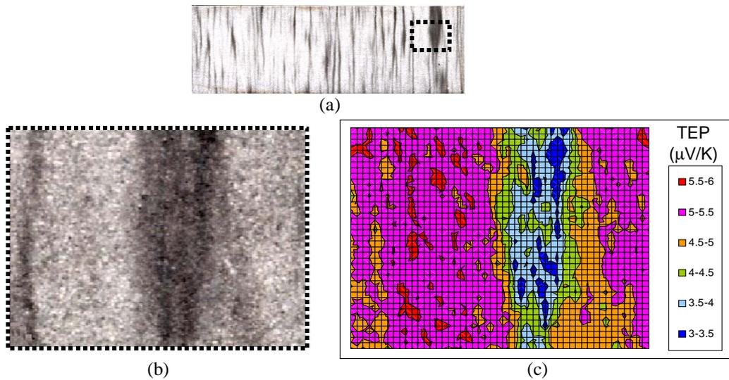
**Figure 6.** (b) Region of a S-sample (a) corresponding to the TEP cartography (c)
