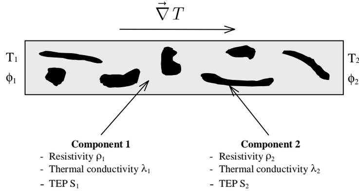
**Figure 2.** Two-dimensional composite sample made up of two different phases
