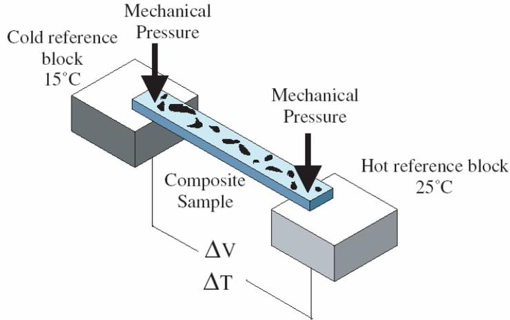
**Figure 1.** TEP (Seebeck coefficient) measurement schema
