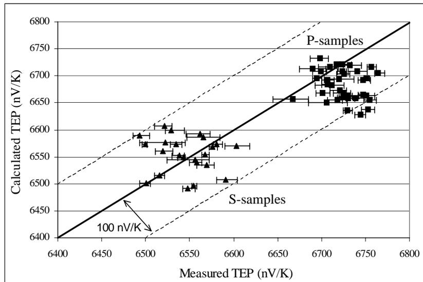
**Figure 8.** Comparison of measured and calculated TEP for ferritic steel samples
