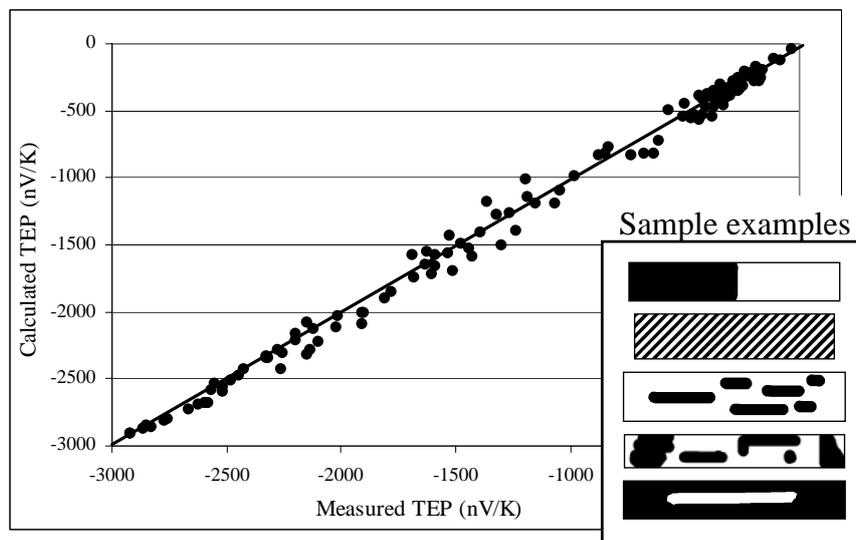
**Figure 4.** Comparison of measured and calculated TEP for Cu/Solder composite samples
