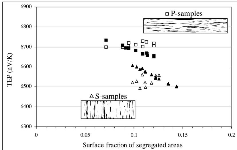
**Figure 7.** Comparison between measured TEP (hollow symbols) and calculated TEP (filled symbols) as a function of the surface fraction of segregated areas
