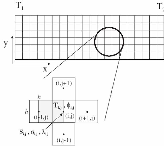
**Figure 3.** Discretization of the composite sample
