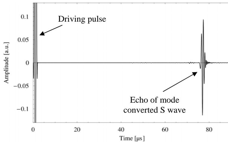
**Figure 9:** Time-domain signal of normal particle velocity according to figure 8, calculated by integrating over the transducer aperture. From the sensor signal the time-of-flight of the mode converted S wave,  $T_S$ , can be determined (step 3 of the prism technique).
