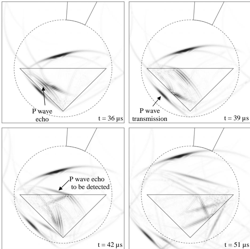
**Figure 6:** 2-D EFIT simulation for a P wave refraction angle of  $45^\circ$  for the water/mortar example (size of the model =  $10 \times 10$  cm, side length of the prism = 5 cm, center frequency of the input pulse = 1 MHz). The wave front snapshots represent the absolute value of particle velocity using a linear grey scale. They were taken at  $t \approx 6, 24, 30, 33, 36, 39, 42,$  and  $51 \mu\text{s}$  after start of excitation.
