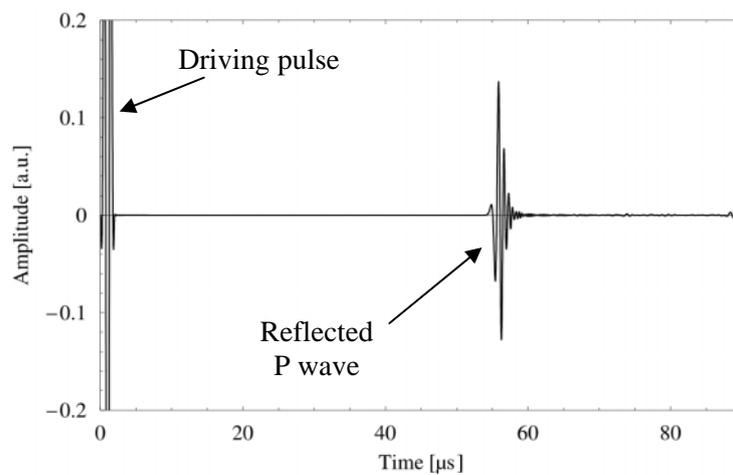
**Figure 5:** Time-domain signal of normal particle velocity according to figure 4, calculated by integrating over the transducer aperture. From the sensor signal the time-of-flight of reflected P wave,  $t_p$ , can be determined (step 1 of the prism technique).
