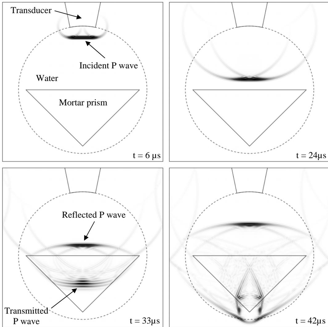
**Figure 4:** 2-D EFIT simulation of normal incidence case for the water/mortar example (size of the model =  $10 \times 10$  cm, side length of the prism = 5 cm, center frequency of the input pulse = 1 MHz). The wave front snapshots represent the absolute value of particle velocity using a linear grey scale. They were taken at  $t \approx 6, 24, 33,$  and  $42 \mu\text{s}$  after start of excitation.
