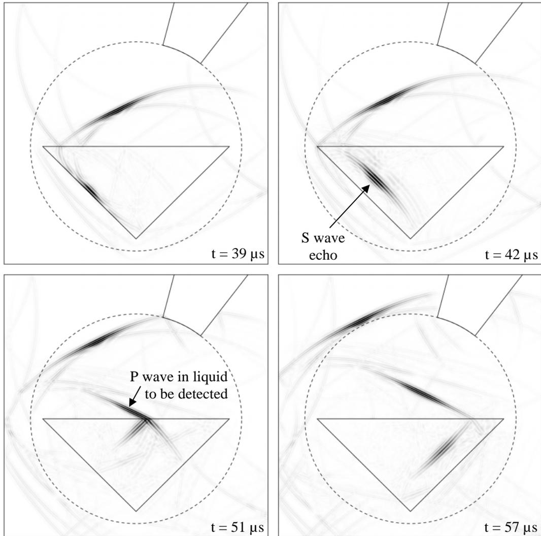
**Figure 8:** 2-D EFIT simulation for S wave refraction angle of  $45^\circ$  for the water/mortar example (size of the model =  $10 \times 10$  cm, side length of the prism = 5 cm, center frequency of the input pulse = 1 MHz). The wave front snapshots represent the absolute value of particle velocity using a linear grey scale. They were taken at  $t \approx 6, 21, 30, 36, 39, 42, 51,$  and  $57 \mu\text{s}$  after start of excitation.
