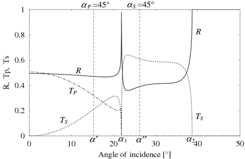
**Figure 2:** Intensity reflection coefficient,  $R$ , transmission coefficient for the refracted P wave,  $T_P$ , and transmission coefficient for the mode converted S wave,  $T_S$ , as a function of the angle of incidence  $\alpha$  for a water/mortar combination ( $\rho_l = 1000 \text{ kg/m}^3$ ,  $c_l = 1470 \text{ m/s}$ ,  $\rho = 2133 \text{ kg/m}^3$ ,  $c_p = 3950 \text{ m/s}$ ,  $c_s = 2355 \text{ m/s}$ ).
