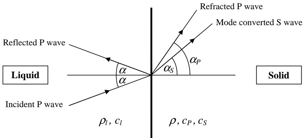
**Figure 1:** Reflection, refraction, and mode conversion of an obliquely incident P wave at a liquid-solid interface.
