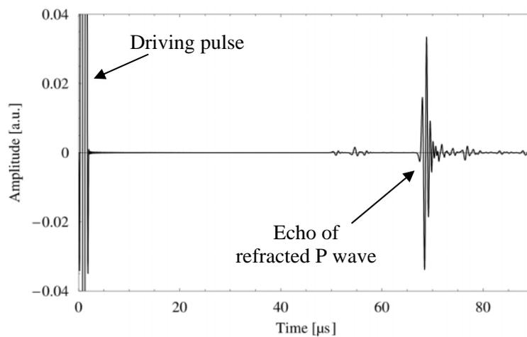
**Figure 7:** Time-domain signal of normal particle velocity according to figure 6, calculated by integrating over the transducer aperture. From the sensor signal the time-of-flight of the refracted P wave,  $T_P$ , can be determined (step 2 of the prism technique).
