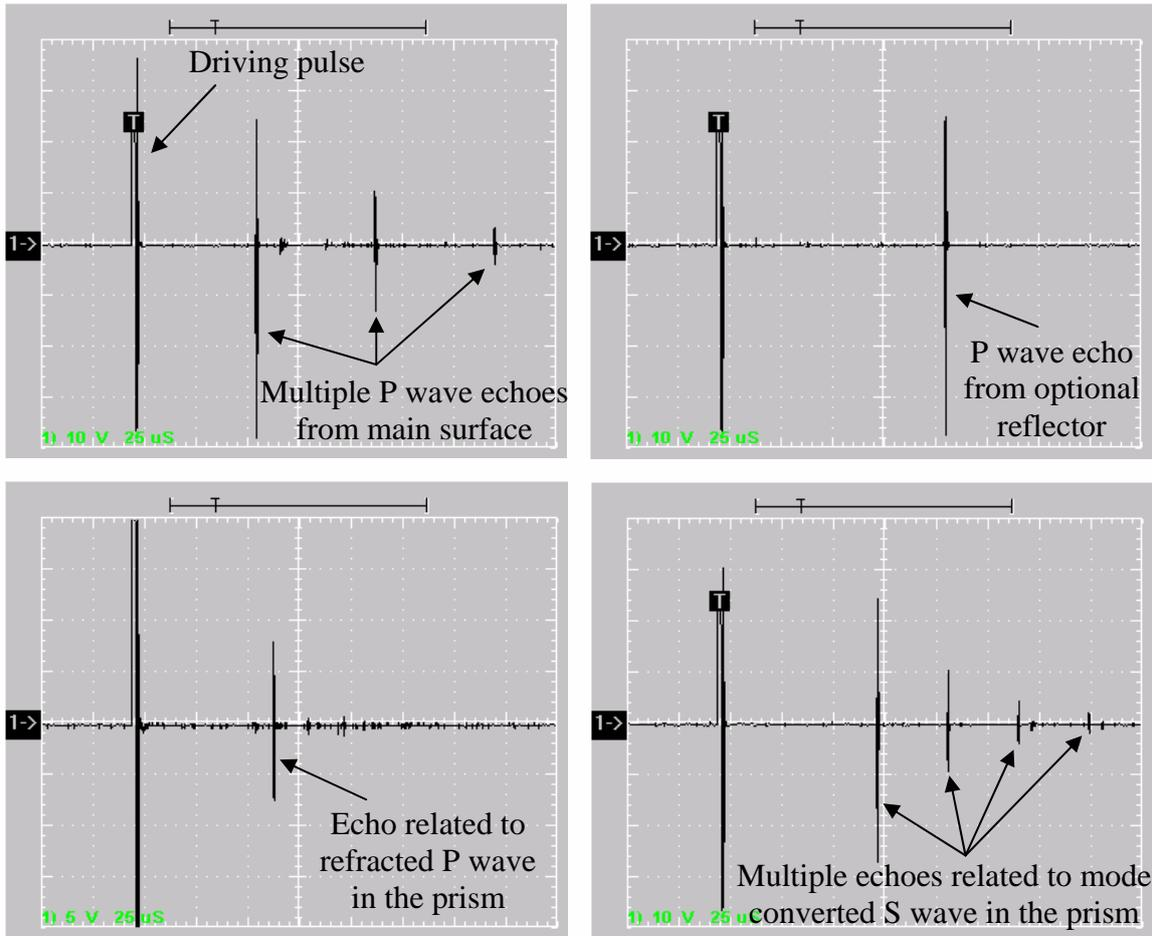
**Figure 11:** Oscilloscope displays obtained for an Aluminum sample showing multiple echoes from the main face of the specimen (top left), an echo from the optional reflector (top right), an echo related to the refracted P wave in the prism (down left), and multiple echoes related to the mode converted S wave in the prism (down right).
