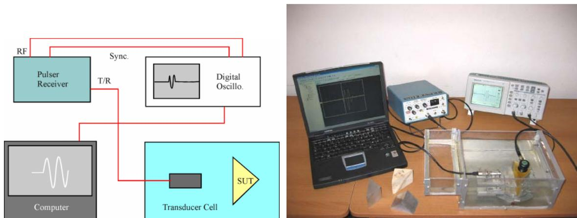
**Figure 10:** Schematic diagram (left hand side) and photograph (right hand side) of the ultrasonic apparatus.
