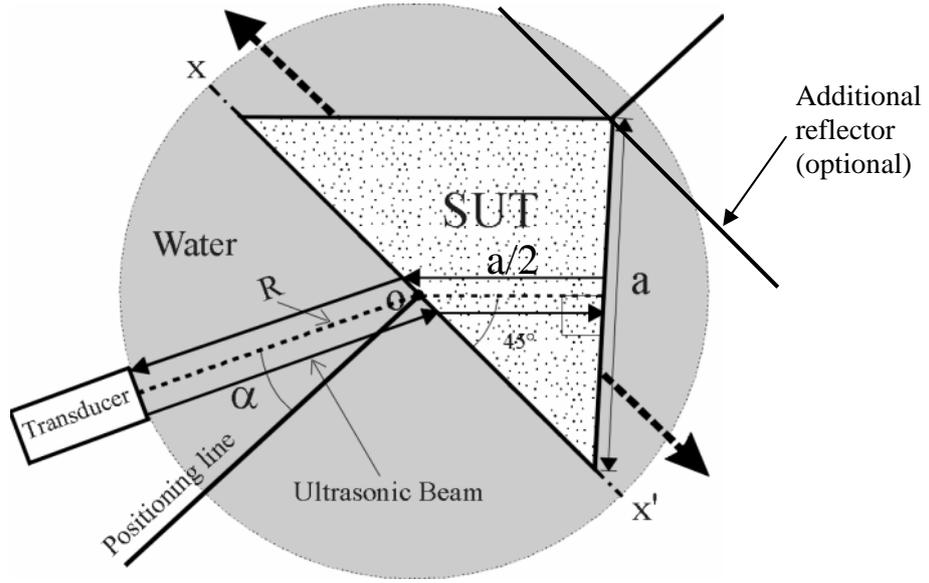
**Figure 3:** Transducer cell configuration as used for the prism technique.
