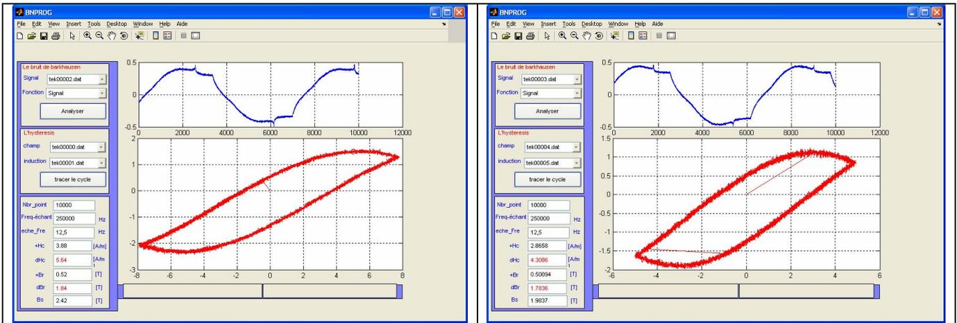
Figure4 : loop hysteresis and BN treated by Software
