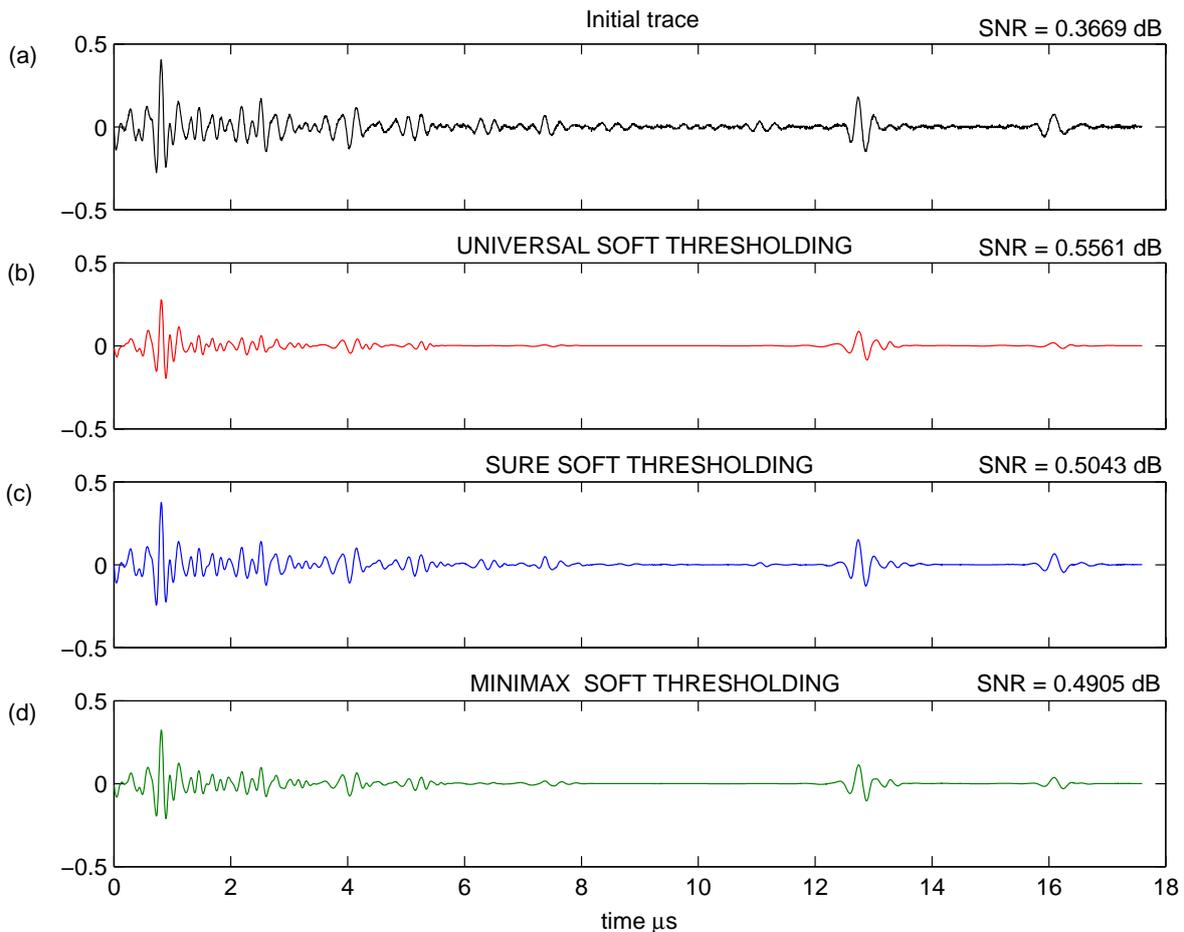
**Figure 4.** Experimental ultrasonic trace (a) and results of de-noising with soft thresholding and different threshold selection rules: Universal (b), SURE (c) and Minimax (d).
