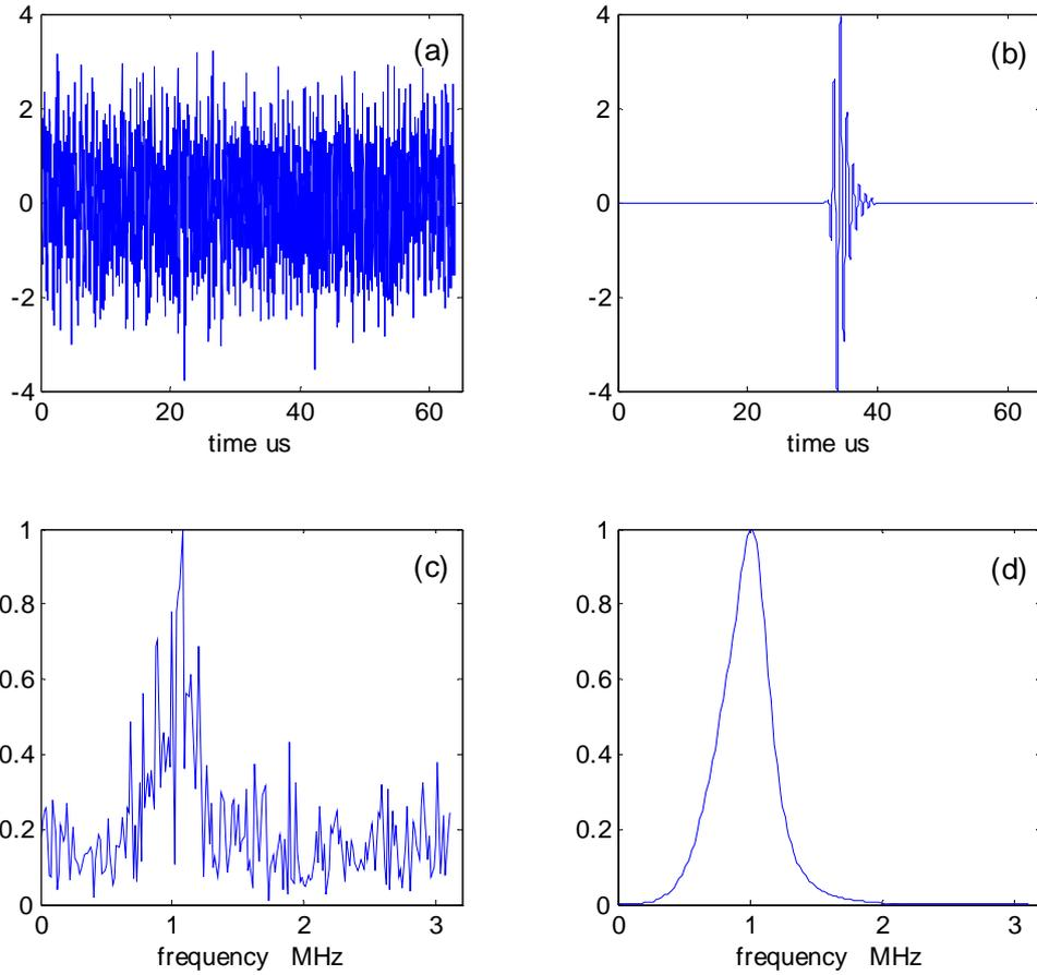
**Figure 2.** Synthetic noise register (a), clean ultrasonic echo (b), and their frequency spectrums (c) and (d).
