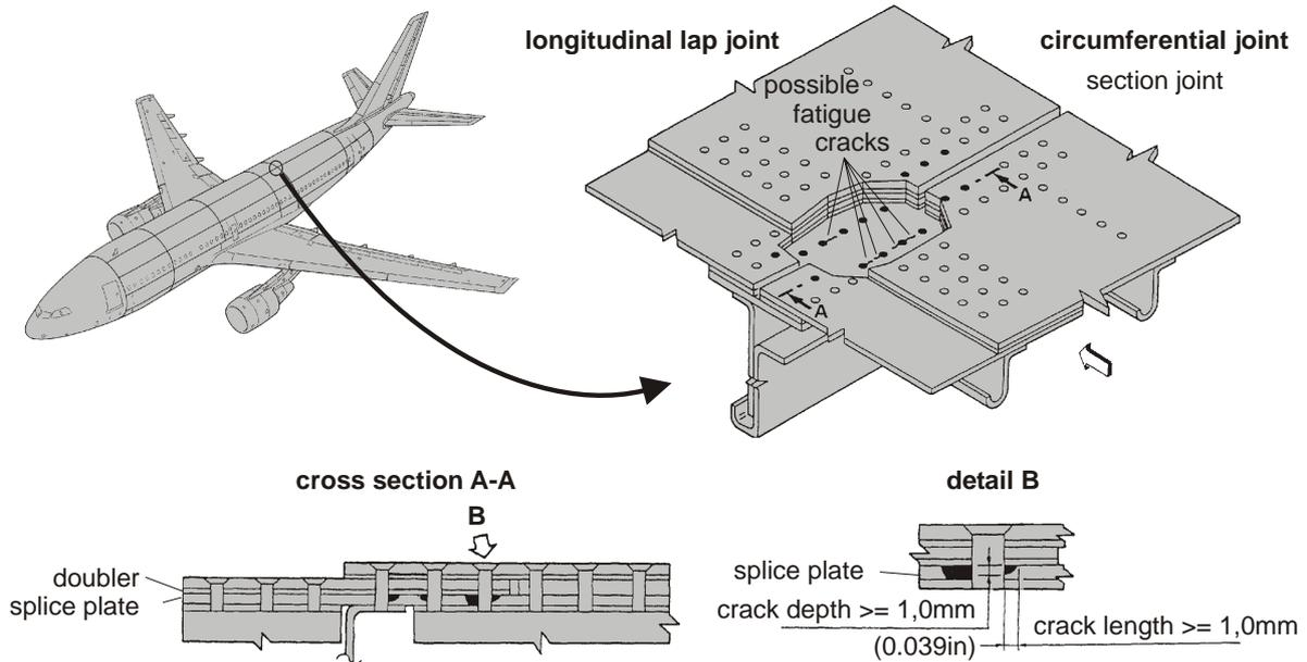
Figure 1 illustrates as example an inspection at the intersection of a longitudinal lap joint and a circumferential joint.
