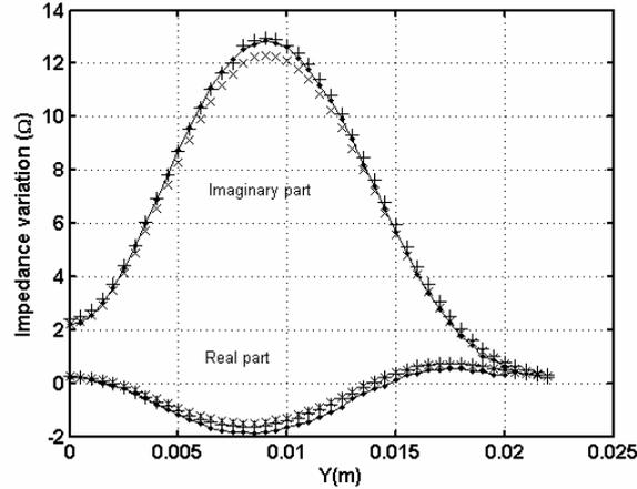
Fig. 7. Variation of the probe impedance:  $\mathbf{a}\text{-}\psi$  (+),  $\mathbf{t}\text{-}\phi$  (x) and experimentation (—).
