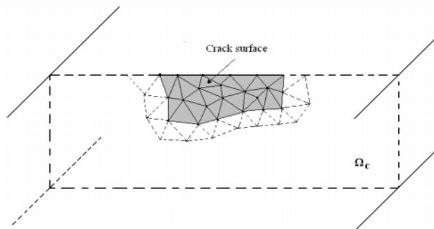
Fig. 3. Crack discretization by finite element facets
