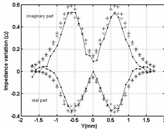
Fig. 8. Variation of the probe impedance (crack: 0.8 mm x 0.1 mm ):  $\mathbf{a}\text{-}\psi$  (+),  $\mathbf{t}\text{-}\phi$  (x) and experimentation (—).
