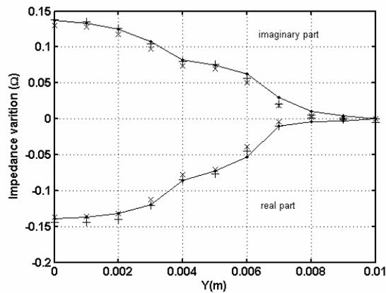
Fig. 6. Variation of the probe impedance  $\mathbf{a}\text{-}\psi$  (+),  $\mathbf{t}\text{-}\phi$  (x) and experimentation (—).
