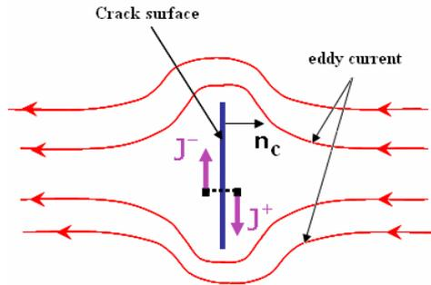
Fig. 2. Effect of the crack on the current density
