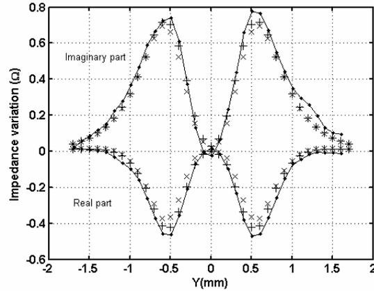
Fig. 7. Variation of the probe impedance (crack: 0.4 mm x 0.2 mm ):  $\mathbf{a}\text{-}\psi$  (+),  $\mathbf{t}\text{-}\phi$  (x) and experimentation (—).
