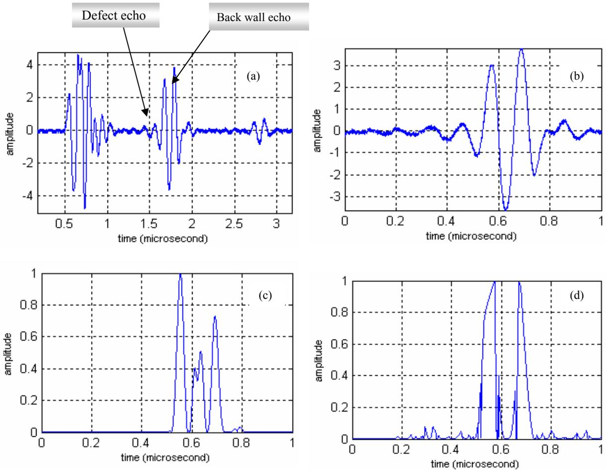
Figure 6. Experimental results. (a) input signal with defect echo closed to back wall echo. (b) defect echo and back wall echo zoomed. (c) result obtained using SSP Q constant and geometric mean. (d) result obtained using SSP Q constant and minimisation
