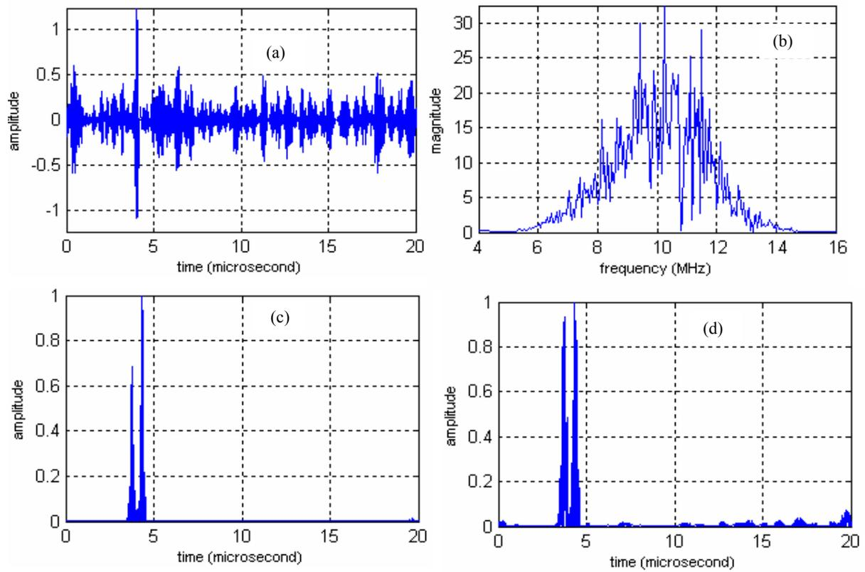
Figure 4.  $2b=5\text{MHz}$  (a) input signal with structural noise (60%) – (b) its spectrum – (c) output signal using SSP with Q-constant algorithm. Geometric mean – (d) output signal using SSP with Q-constant algorithm. Minimisation
