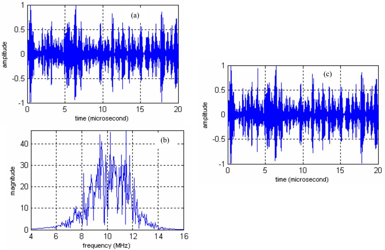
Fig.1.(a) Modelled noise, (b) Noise spectrum
