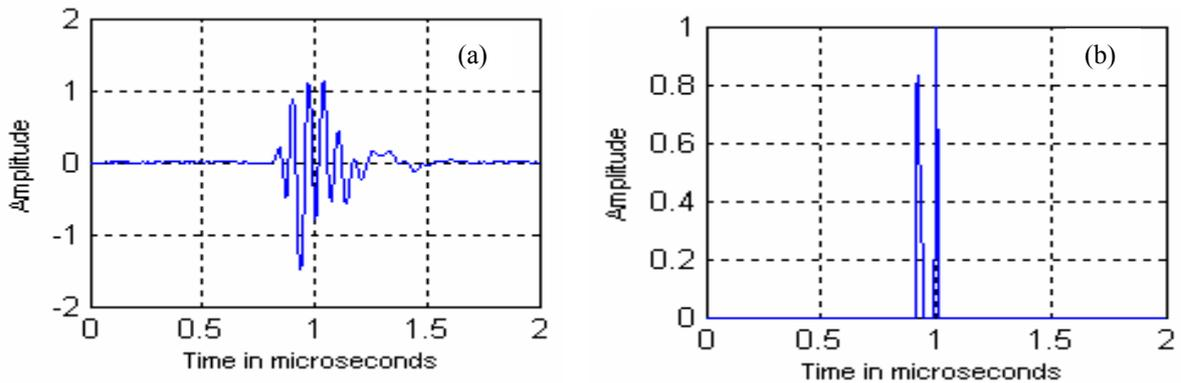
Figure 7. Experimental results of composite material. Thickness=0.6mm,  $f_c=15$  MHz (a) input signal with front echo closed to back wall echo. (b) result obtained using SSP Q constant and minimisation ( $Q = 5$ , 1<sup>st</sup> filter location= 3 MHz, last filter location= 11Mhz, Number of filters = 12).
