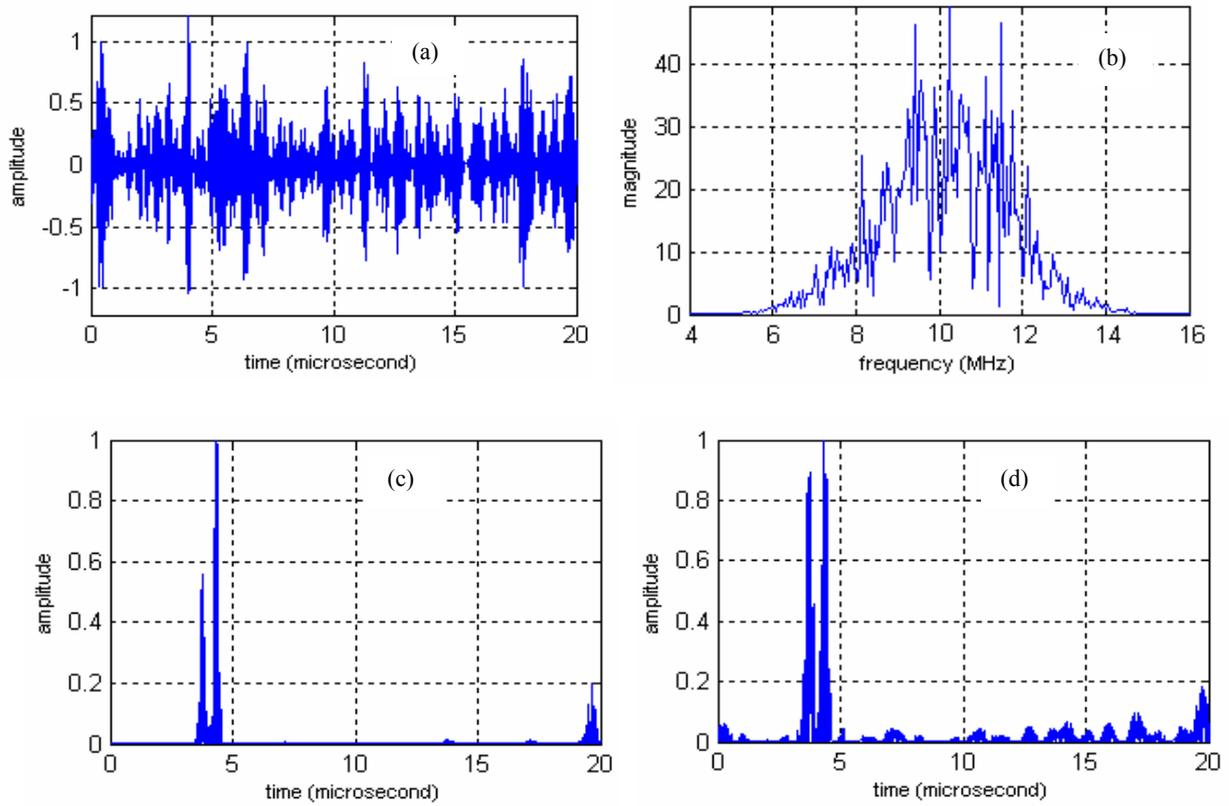
Figure 5.  $b=2.5\text{MHz}$  (a) input signal with structural noise (100%) – (b) its spectrum – (c) output signal using SSP with Q-constant algorithm. Geometric mean – (d) output signal using SSP with Q-constant algorithm. Minimisation
