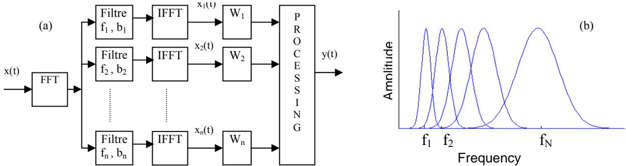
Fig.2. (a) Filter bank of SSP. (b)  $Q$  constant bandwidth of filters
