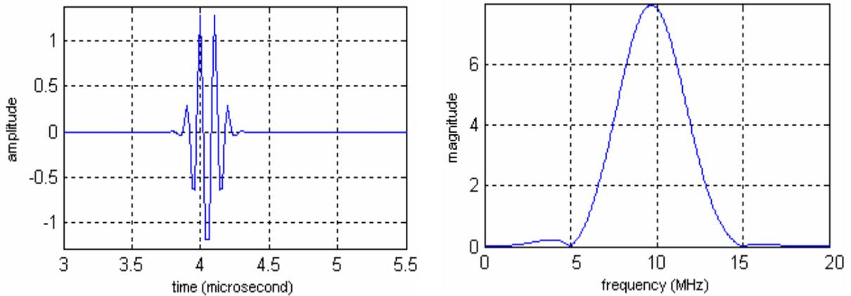
Figure 3. (a) Free noise input signal with two echoes separated by  $\Delta t = 0.1 \mu\text{sec}$ .
