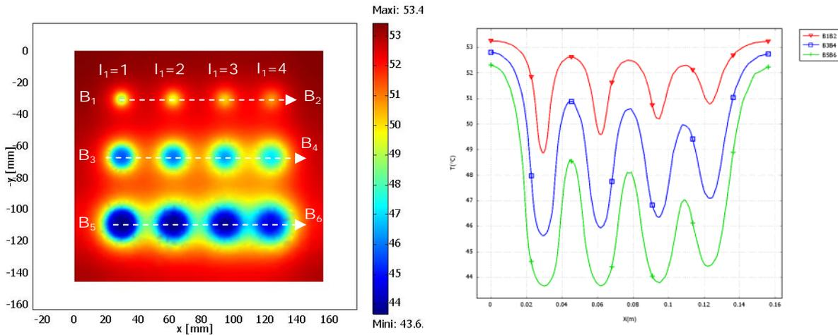
**Figure 8.** Influence of defect position on the entry surface temperature profile along the lines ( $\nabla$  :  $B_1B_2$ ,  $\square$  :  $B_3B_4$ ,  $+$  :  $B_5B_6$ )
