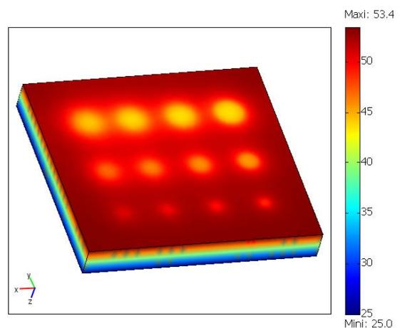
**Figure 6.** Temperature distribution in the wall with defect
