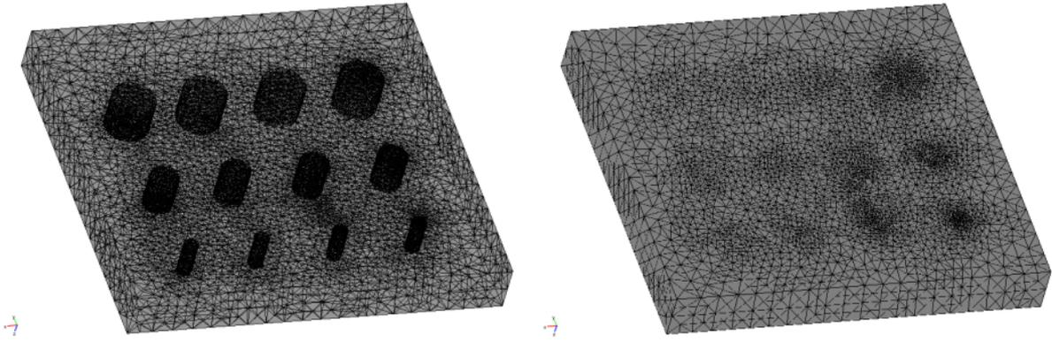
**Figure 4.** Mesh of the wall with 12 defects
