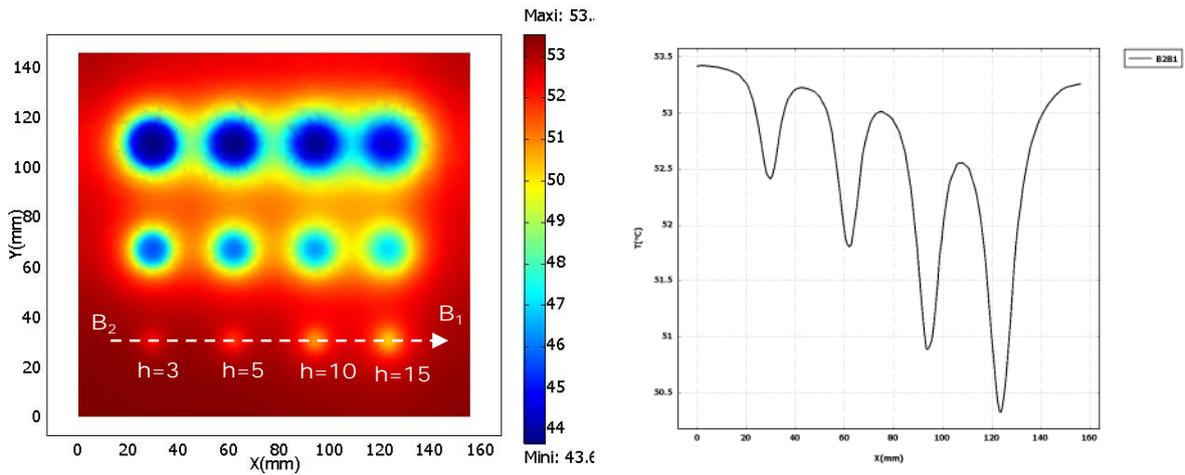
**Figure 10.** Influence of defect thickness on the entry surface temperature profile along the line ( $B_2B_1$ ,  $l_1=2$ mm,  $h=3, 5, 10,$  and  $15$ mm)
