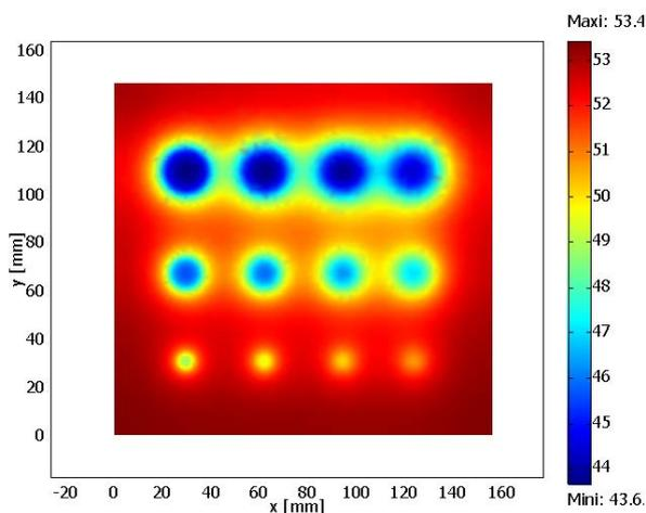
**Figure 5.** Temperature distribution on the front face of the wall with defect
