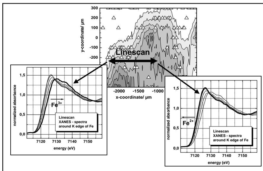
Fig. 2: Elemental micro-XRF mapping in combination with a micro-XANES linescan. The micro-XRF mapping showed here indicates higher relative concentrations of Zn in the edge region of the ink (white triangles plotted in the Fe concentration profile) and therefore a higher mobility of Zn. The micro-XANES line scan indicates an increasing  $\text{Fe}^{2+}$  concentration with increasing ink area density
