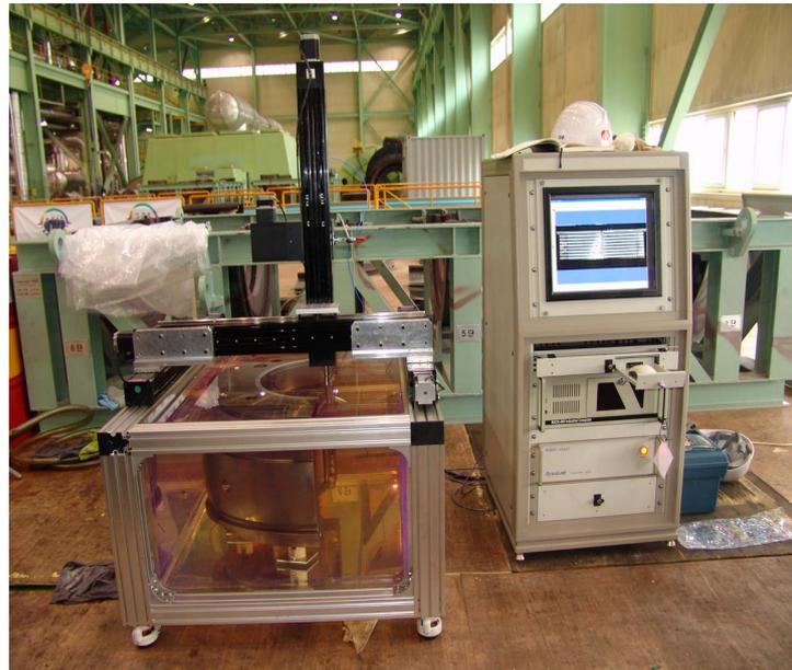
**Fig. 2** Field set up of C-Scan equipment
