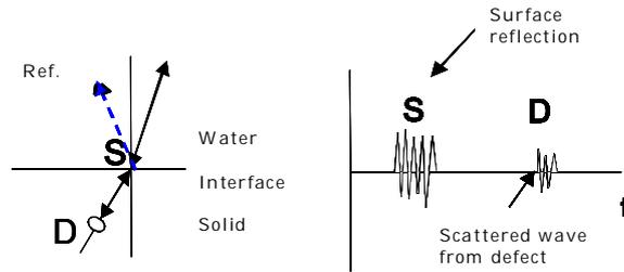
**Fig.2.** Backscattering model of mode-converted transverse wave.
