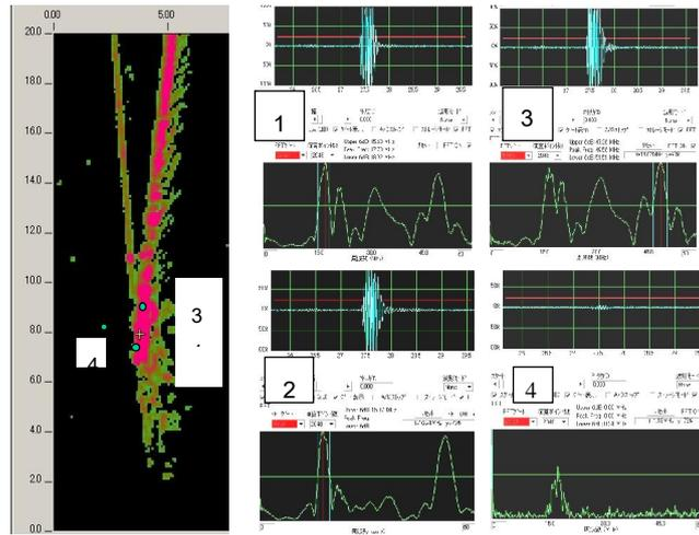
**Fig. 9** Higher harmonic images of fatigue-cracked surface. Incident wave: 17MHz, 2<sup>nd</sup> harmonic: 34MHz, 3<sup>rd</sup> harmonic: 51MHz. Frequency range: 0- 60MHz.
