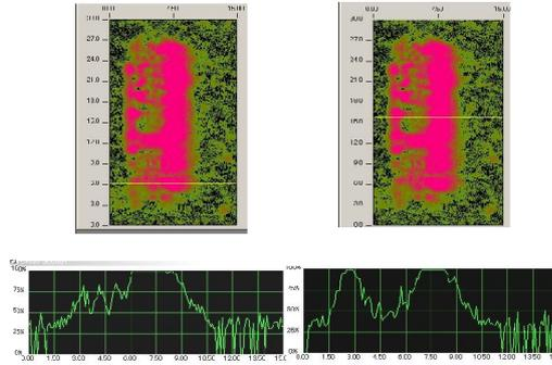
Fig.7 Fatigue crack surface image. Transducer:30MHz, F=25mm.
