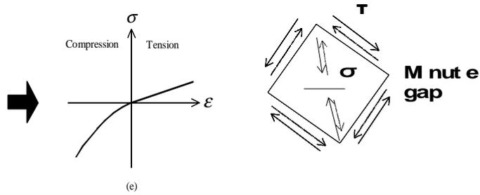
**Fig. 4** Clapping of crack surface under transverse wave.
