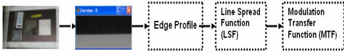
Figure 1: Schematic of concept for MTF determination using ESF
