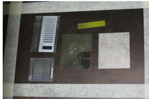
Figure 3: Test object for image quality assessment
