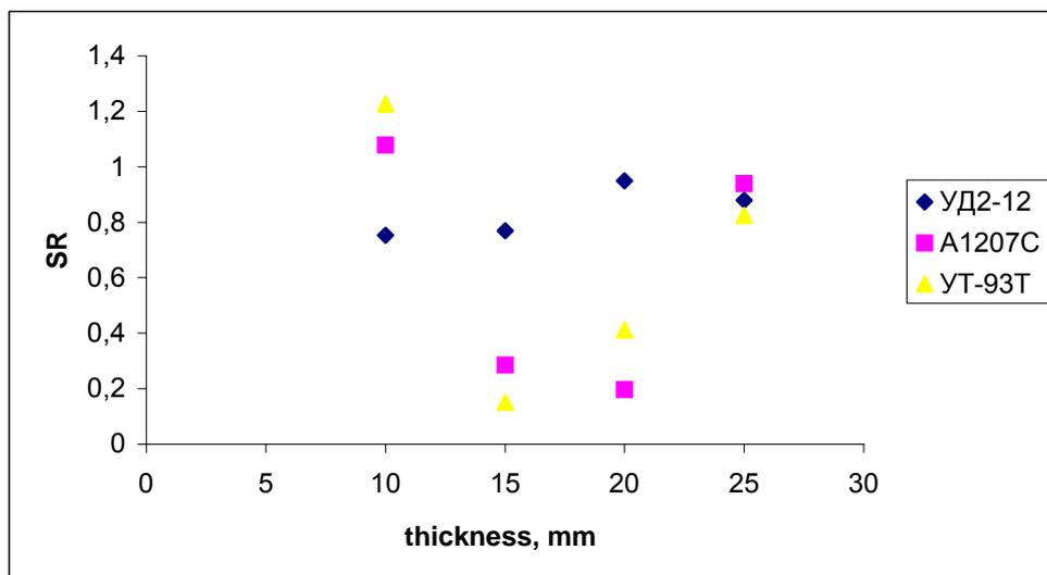
**Figure 3:** Reproducibility of thickness measurements of metal structure components by thickness gauges of various types
