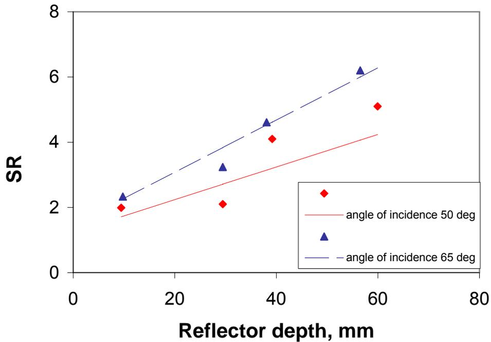
**Figure 1:** Reproducibility of reflector depth measurements (11 operators 10 measurements each)
