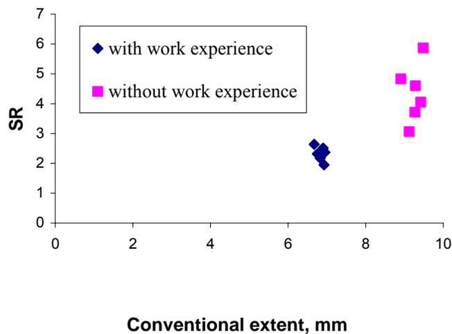
**Figure 2:** Reproducibility of conventional extent measurements for vertical cylindrical holes (10 operators, from 5 to 8 measurements)
