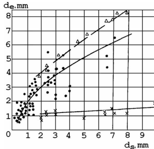
Figure 1. Correlation between of equivalent diameter  $d_e$  and its true size  $d_s$ : • - volumetric defects; x, Δ - cracks at measurement with single ultrasonic probe and under the "tandem", respectively [3].
