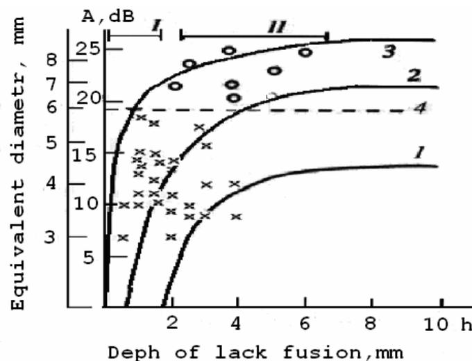
Figure 2. Dependence of echo-signal amplitude on the depth of lack of penetration (nonpenetration) for a single probe ( $f = 2,5$  MHz, and  $\beta = 30^\circ$ ) [4].
