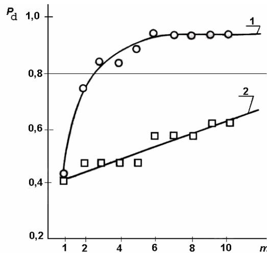
Figure 4. Dependence of the defect detection on the number of testings (1) carried out by different NDT Inspectors (2) [5].
