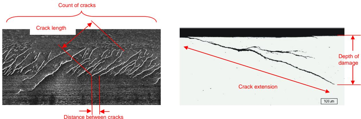
**Figure 1:** Head check cracks
