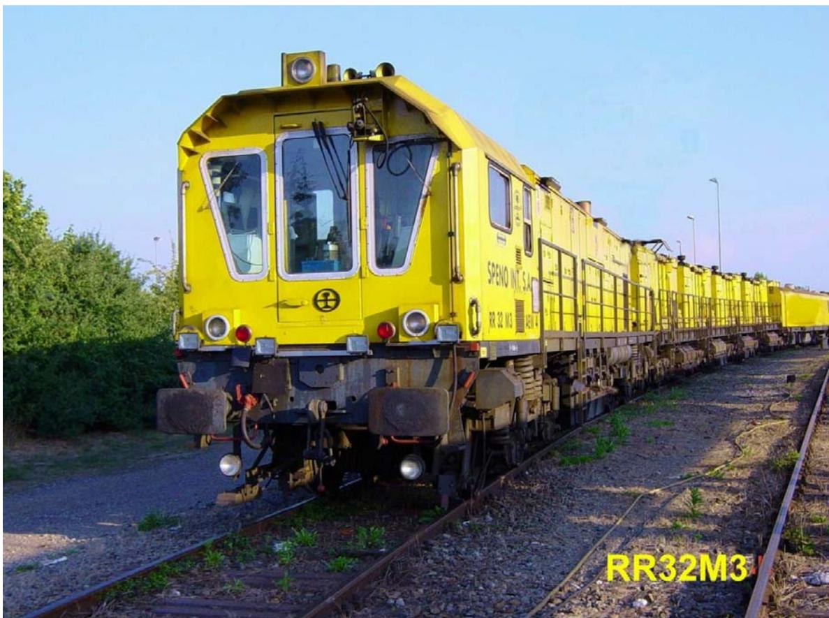
**Figure 2:** Grinding machine train
