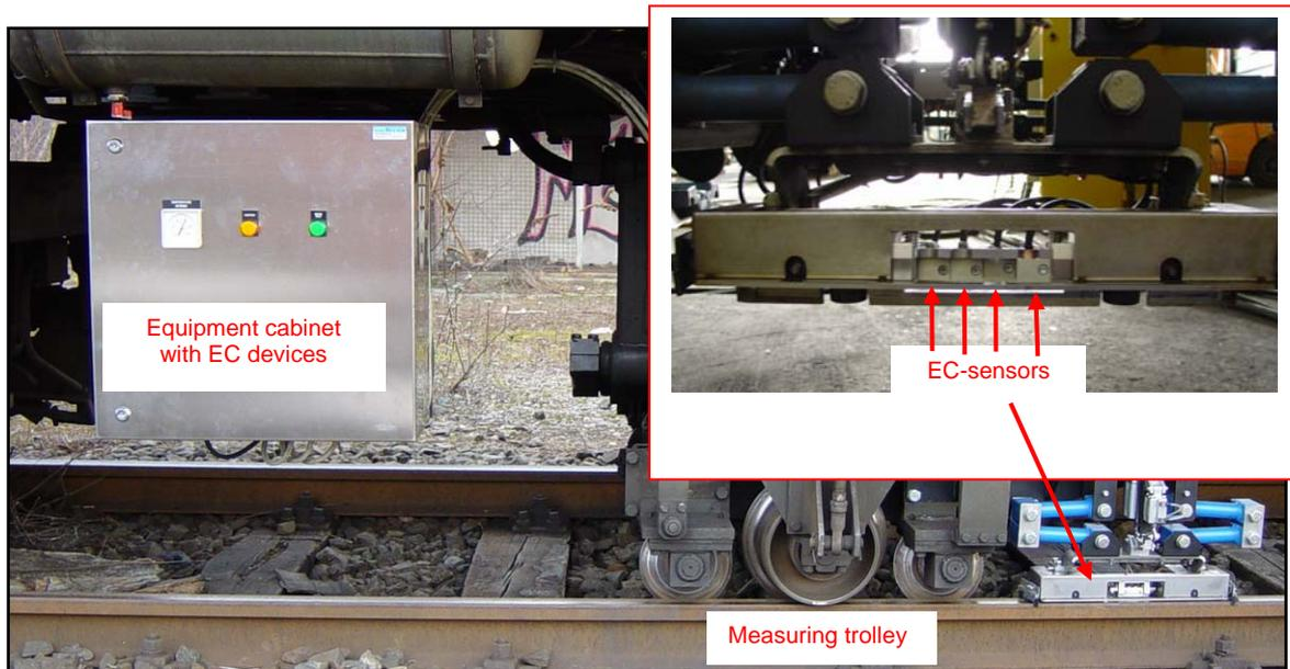
**Figure 3:** Measuring system under the grinding train
