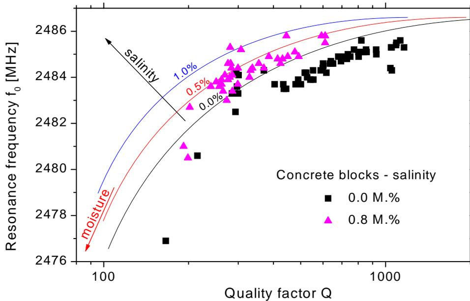
Fig. 11. Measured quality factor  $Q$  and resonance frequency  $f_0$  of concrete blocks of different salinity, measured with the 2.45 GHz resonator during drying. For comparison, the contours of constant salinity are drawn as thin lines.
