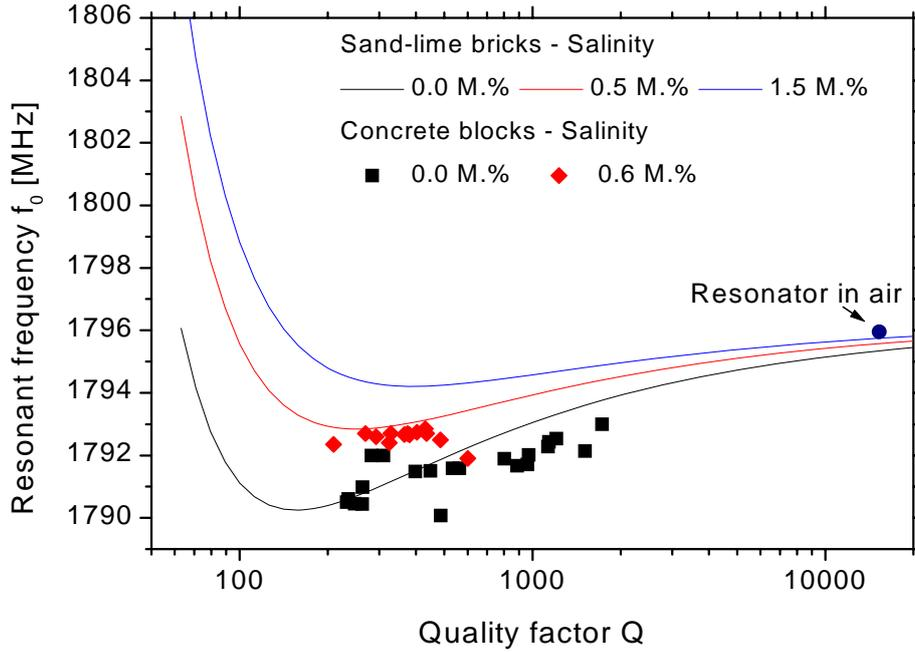
Fig. 10. Measured quality factor  $Q$  and resonance frequency  $f_0$  of concrete blocks of different salinity. The data were measured with the 1.8 GHz resonator at different times during the drying period (variable moisture). For comparison, the contours of constant salinity are also given.
