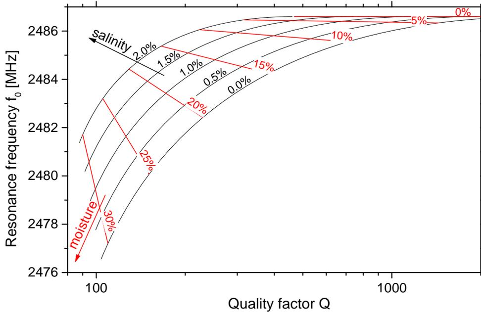
Fig. 9. Contours of constant moisture and of constant salinity in a graphical representation of the resonant frequency and the quality factor of the resonance of the dielectric 2.45 GHz resonator.
