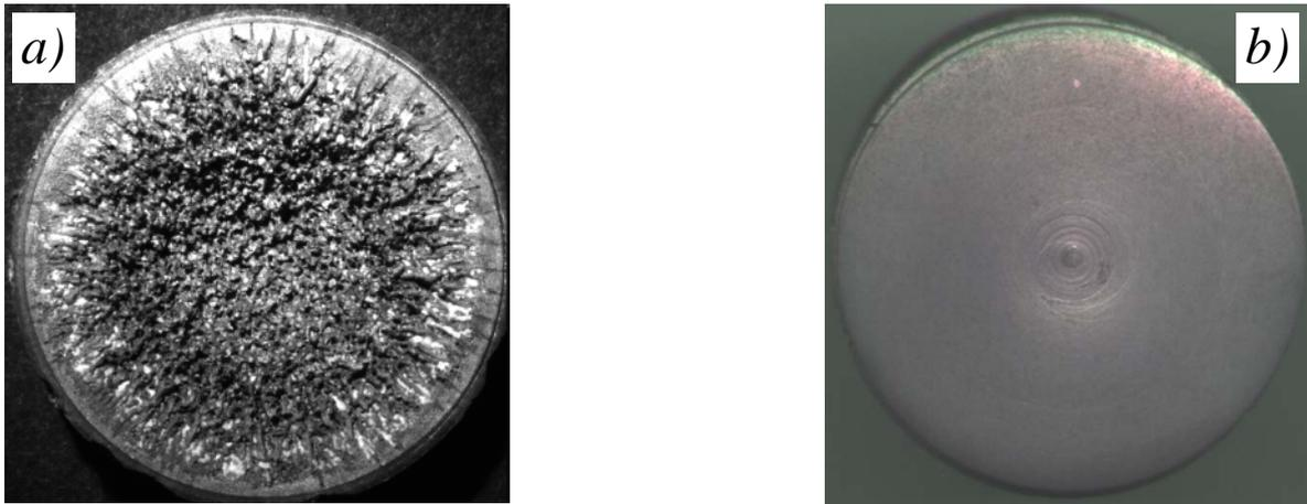
Fig. 4. Micrograph images of the surfaces of the horn like end piece after 500 h functioning: *a)* Duraluminum unprotected; *b)* Stainless steel protected
