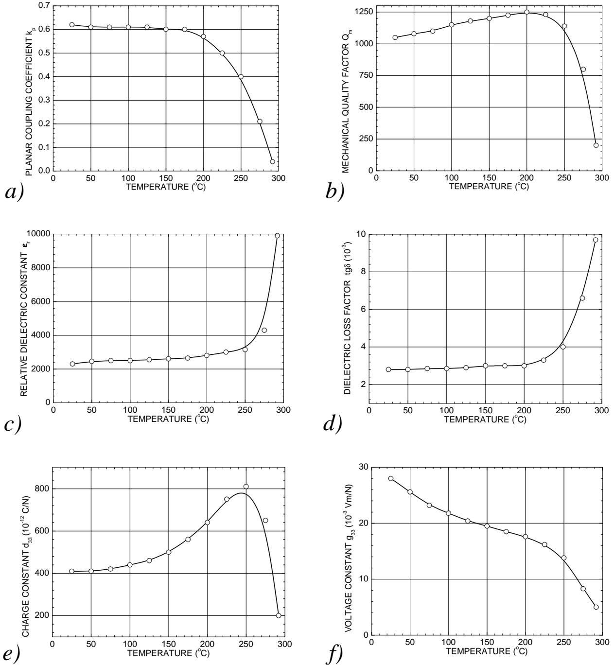
**Fig. 2.** The temperature dependence of the main piezoelectric parameters of the piezoceramic material:
