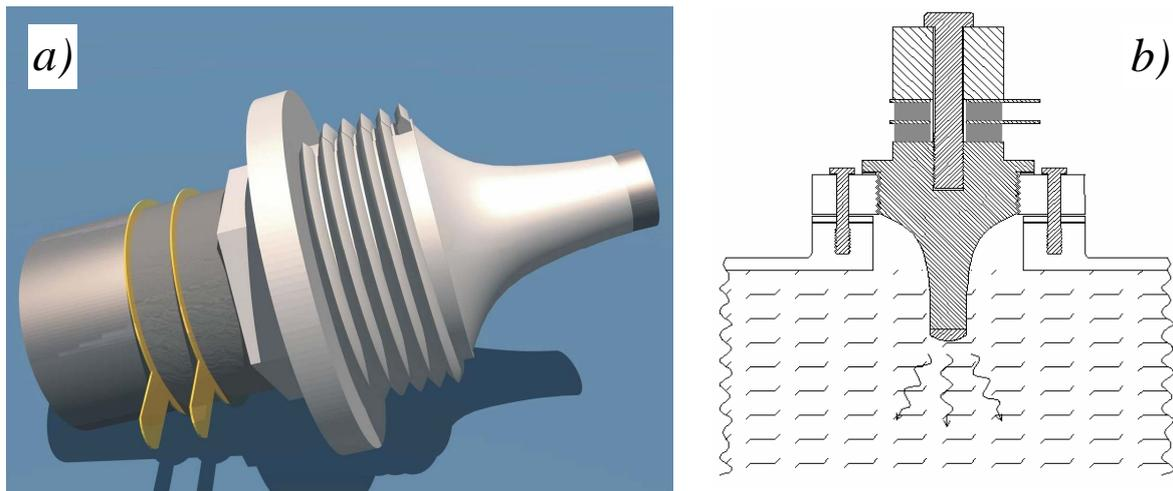
**Fig. 3.** Piezoceramic transducer: *a)* General view; *b)* Mounted in the heat exchanger
