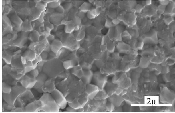
**Fig. 1.** Fracture SEM image of a typical material sample sintered at 1200 °C for 6 hours
