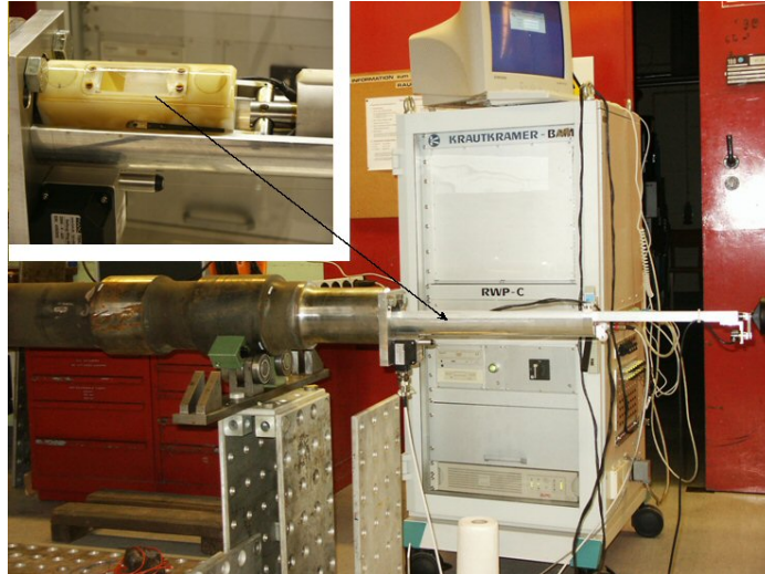
Fig 5 Measuring system for testing axles with bore holes using phased array technique
