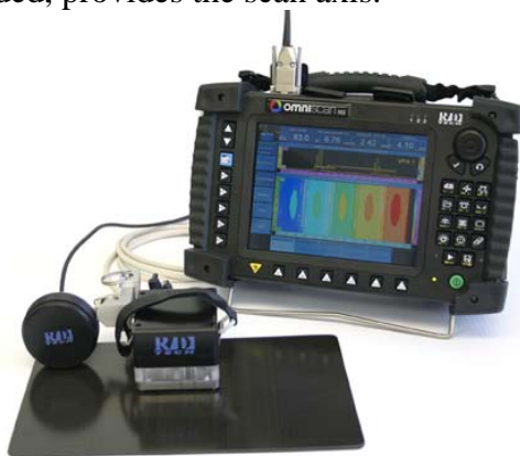
Figure 7. Encoded 128 element probe shown with water box for electronic linear C-Mode imaging of composites
