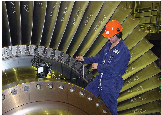
Figure 5. Portable Phased array instrument for multi-angle rotor inspection illustration
