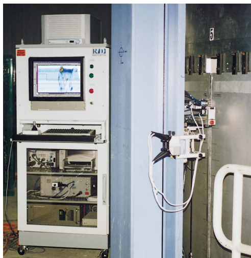
Figure 4. Industrial Phased Array systems for friction stir weld inspection
